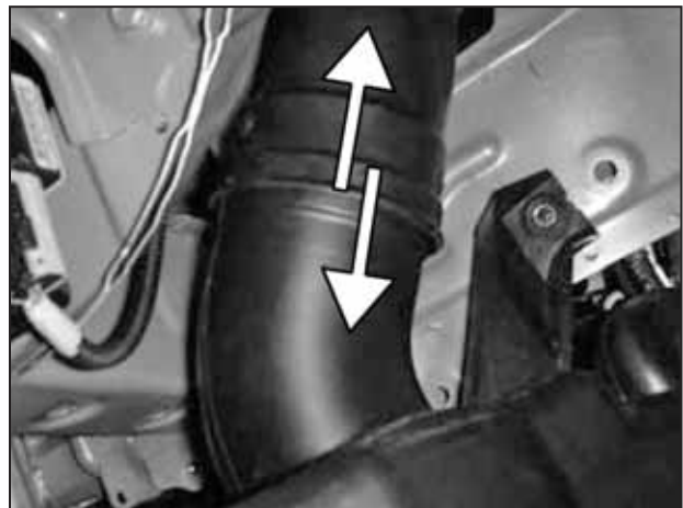
o. Pull the inlet tube off of the resonance chamber and remove the chamber from the vehicle.
