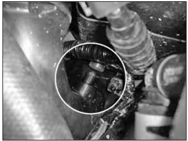
k. Pull the upper inlet tube out of the grommet, located on the side of the battery box.
