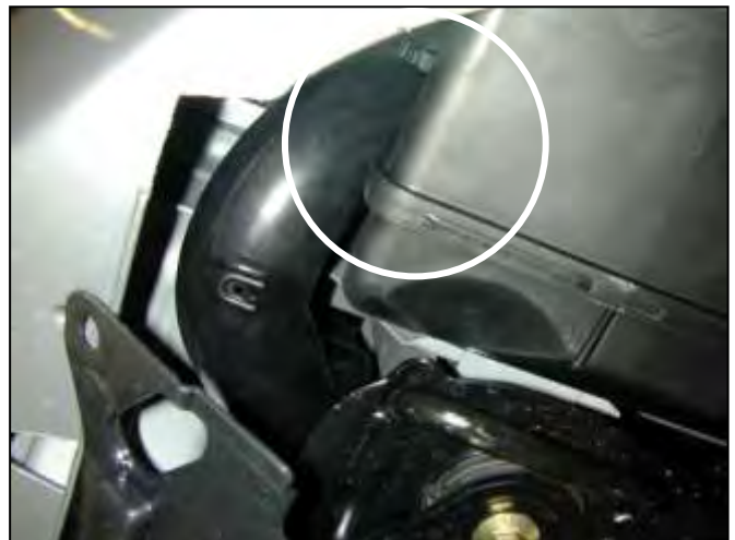
n. Reach up inside the space in front of the resonator assembly with a 10mm socket or wrench and remove the other mounting bolt.
