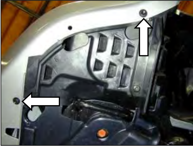
i. From underneath the vehicle, remove the fasteners shown in the image.
