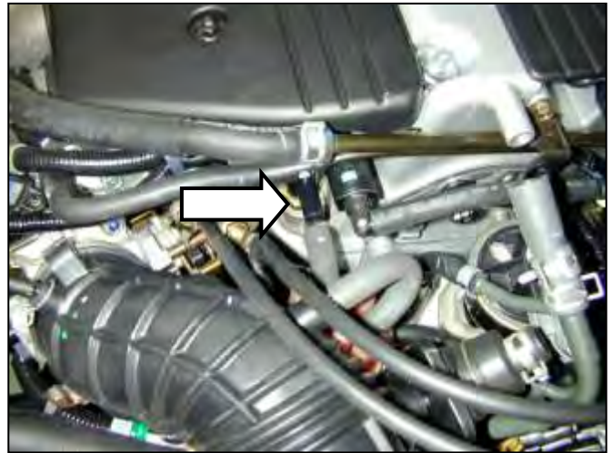
b. Unplug the breather tube from the fitting underneath the intake manifold.
