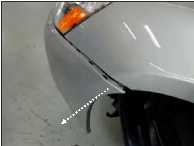
m. Unsnap the corner of the bumper cover as shown in the picture. This will help with the removal of the resonator assembly.
