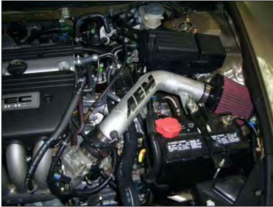
AEM® intake system installed
