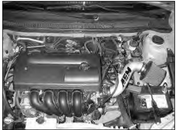
AEM® intake system installed
