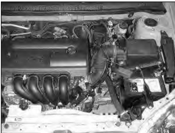
Factory air box system installed
