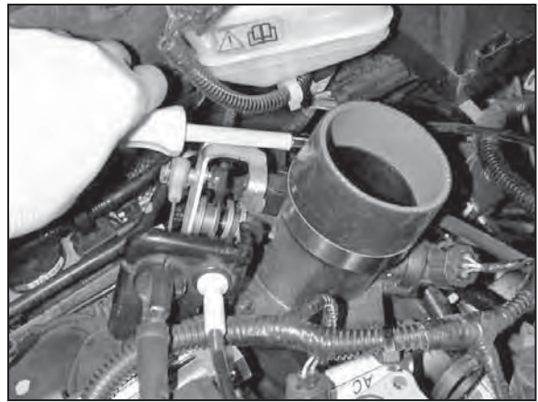
c. Install the 2.75" connector hose on the throttle body using the supplied hose clamps.
