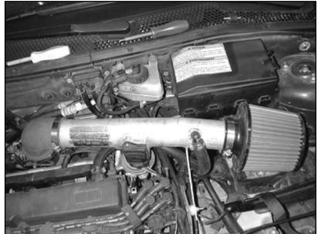
AEM ® intake system installed
