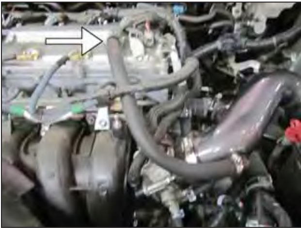
l. Attach the other end of the hose onto the PCV vent and secured it with a supplied hose clamp (# 99024.032).
