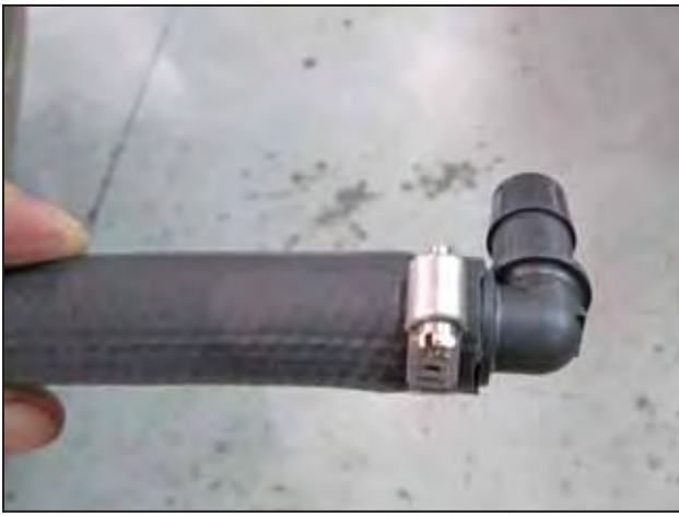
j. Slide the 5/8" hose over the 90° plastic elbow and secure it with the hose clamp (# 99024.032).
