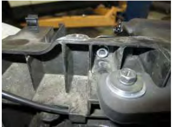
AA. Secure the M6 bolt installed in the previous step by attaching one M6 nut (#4) to the end of the bolt that passed through the radiator support.
