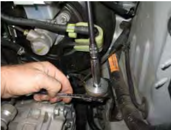
H. Once properly assembled, tighten the nuts and bolts to secure the adapter assemblies.
