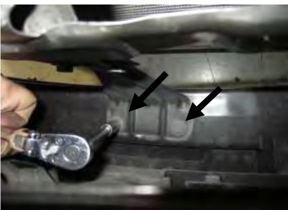
O. Now remove the two 6MM bolts on the bottom of the grill support.
