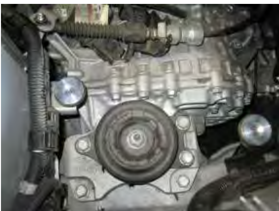
D. Place the two adapters (#10) onto the factory rubber grommets as shown.
