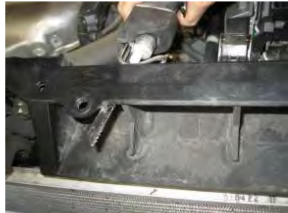
T. Cut the radiator support to make room for the AEM front scoop.
