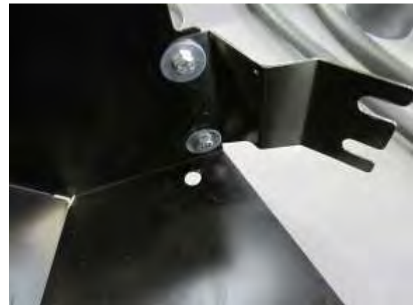
I. Attach the provided bracket (#14) onto the heat shield using two M6 bolts (#7) and two washers (#5).
