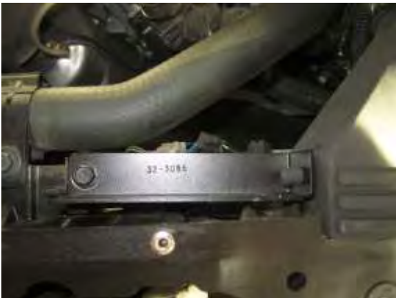
T. Attach bracket (#13) to the air inlet hose and to the radiator support using the provided M6 bolt (#15).
