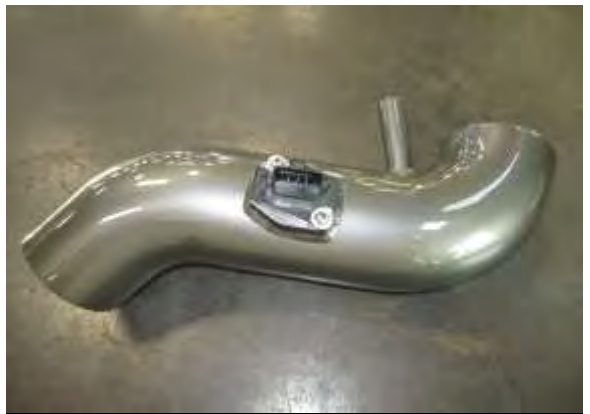
AC. Install the MAF sensor onto the intake tube (#21) using the OEM screws.
