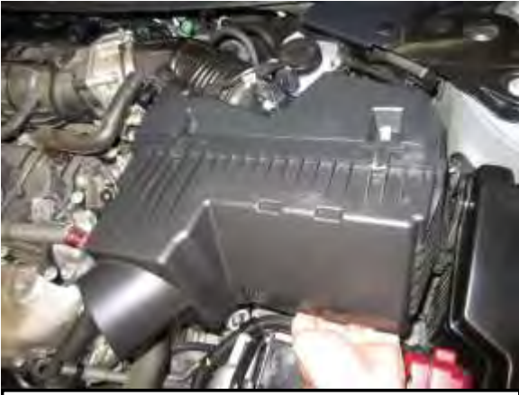
K. Lift up on the bottom of the air box to disengage but do not remove from engine bay.
