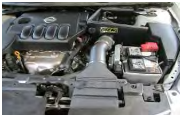
AEM intake Installed
