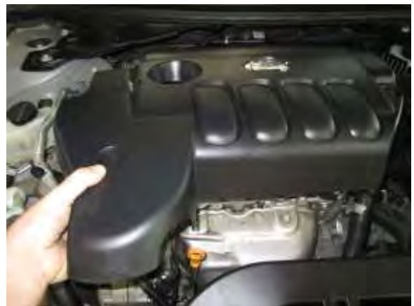
B. Lift up on the bottom of the engine cover and remove it from the vehicle.
