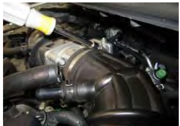
J. Loosen the hose clamp that secures the Inlet tube to the throttle body.
