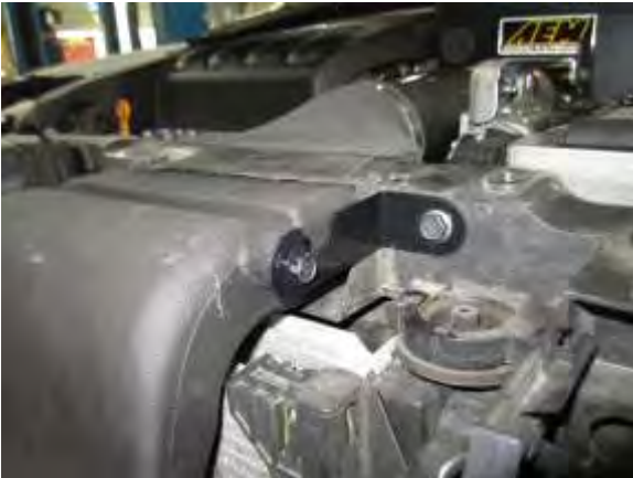
Z. Secure the air inlet scoop's bracket to the radiator support using one M6 bolt (#15).
