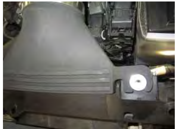
U. Install the mounting block (#9) onto the air inlet hose as shown.
