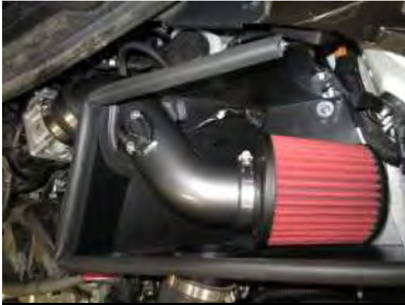
AF. Mount the AEM air filter ( #20) onto the intake tube and secure using a (#22) hose clamp.
