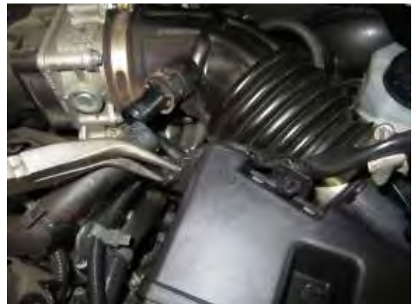
H. Release the two clips securing the MAF sensor harness to the air box.
