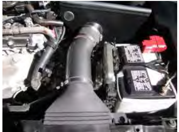
S. Install the air inlet hose assembly into the engine bay as shown.
