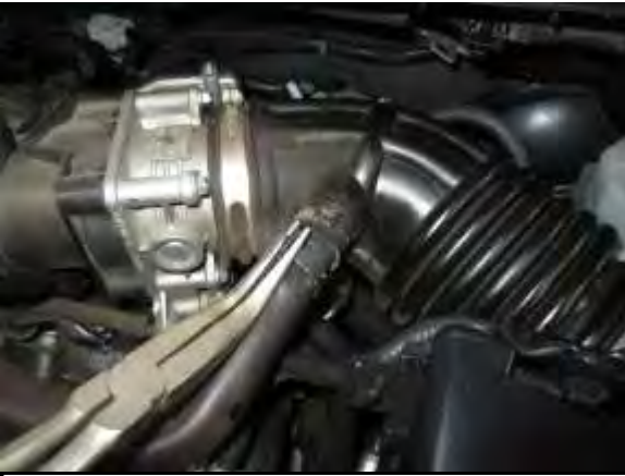
E. Remove the spring clamp securing the PCV hose to the stock intake tube.
