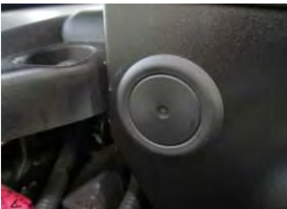
J. Insert the rubber plug (#26) into the heat shield hole as shown.
