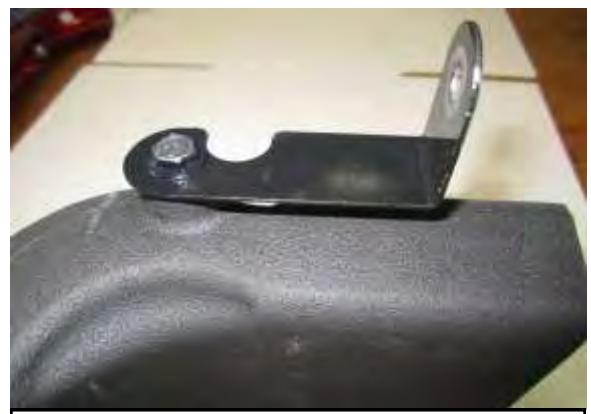
W. Mount the bracket (#19) to the air inlet scoop (#18) using one M6 bolt (#15).
