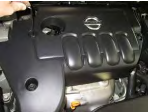
A. Remove the three Allen head bolts that secure the valve cover in place.
