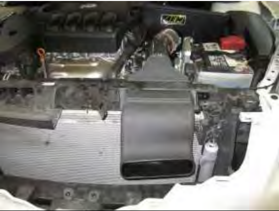
X. Install the air inlet scoop into place as shown.
