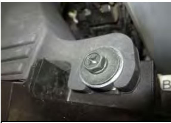
V. Secure the air inlet hose using the OEM bolt and washer (#5) as shown.
