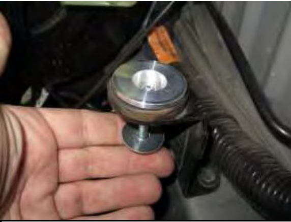
F. From underneath the factory rubber grommets slide each bolt and fender washer through so the bolt protrudes through the rubber grommet and adapter as shown.
