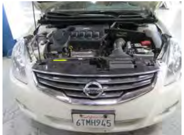
AM. Re install the grill using the factory clips removed in step M.
