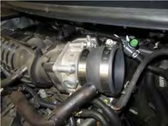
B. Install coupler (#23) onto the throttle body and mount the (#22) and (#24) hose clamps as shown.
