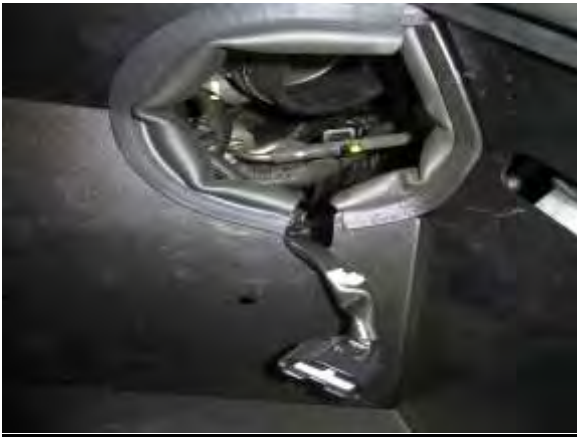
AD. Feed the MAF sensor wire harness into the inside area of the heat shield as shown.
