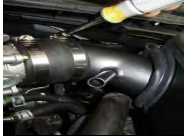
AG. Align the intake pipe with the throttle body's coupler and secure the (#22) hose clamp.
