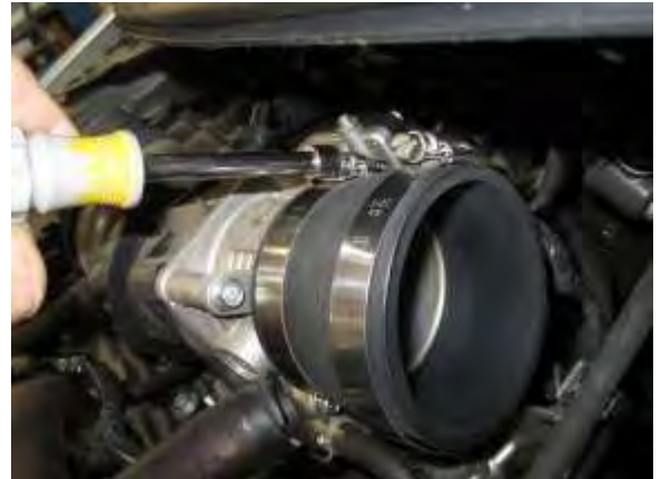
C. Tighten the (#24) hose clamp on the throttle body end.
