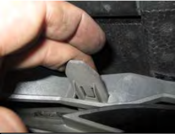
Q. on the back side of the grill, there are clips holding the grill in place. Push in each clip one at a time and push the grill forward. Repeat that on all the clips
