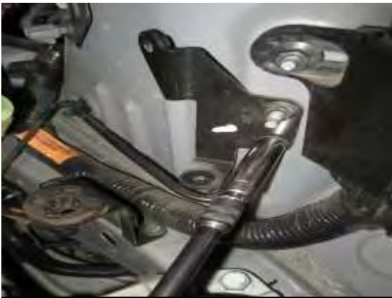
S. Remove the two 6MM bolts securing the factory air box bracket to the inner engine bay wall.
