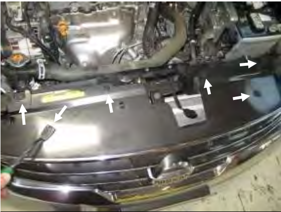
M. Remove the six clips on the top of the front grill.
