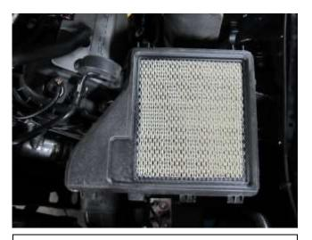
g) Remove the stock filter from the air box.
