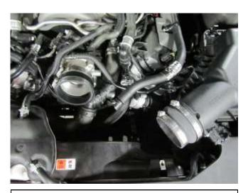
c) Install the couplers onto the throttle body (08654) and the air box (5-1083) with the provided hose clamps (9456).
