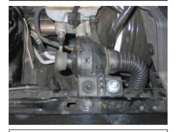
g) Slide the Caplug (08246) over the engine pulse drum as shown.
