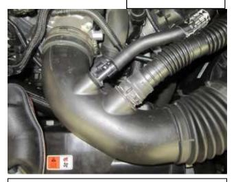
b) Disconnect the engine pulse tube by squeezing the clamp and sliding it off the intake tube. Slide the grey indicator on the valve cover breather hose and detach it from the intake. **Note:** On automatic transmission vehicles, their will be an additional vent line. Depress the yellow tab and slide the line off.
