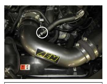
f) Attach the valve cover breather hose by sliding it over the fitting. On automatic transmissions also attach the second hose removed in 2b) to the lower fitting. **Note:** Make sure you hear it click as it attaches to the fitting.
