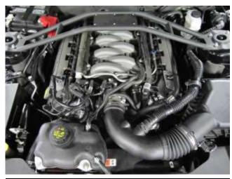
a) Remove the engine cover by lifting up and pulling it out of the vehicle.
