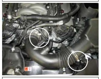
d) Loosen the two hose clamps at the air box and throttle body and remove the stock intake tube.
