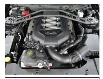
Factory air box system installed
