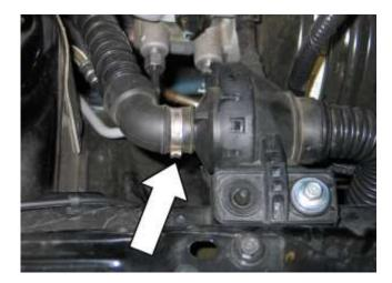
c) Cut the clamp that secures the engine pulse hose to the drum and disconnect the hose from the drum.
