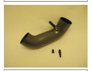
d) Screw in the fitting (082628) into the top port. For the bottom port reference your transmission below:
