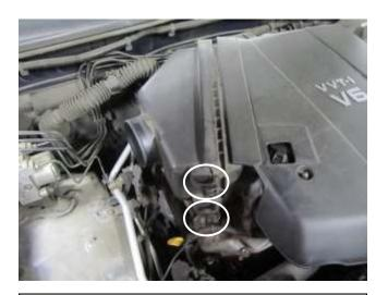
d. Unclip the two stock air box clamps.
