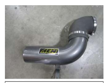
f. Install the 90 degree coupler onto the intake tube with the supplied hose clamps. Do not tighten at this time.
