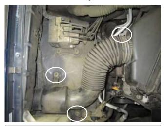
a. Loosen the hose clamp at the air box inlet and remove the two m8 bolts. The bolts will not be reused.
