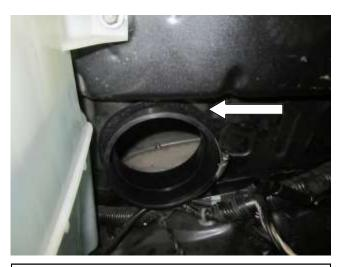
e. Install the edge trim (8-4108) onto the fender. Then squeeze the air accelerator while installing it into the fender with the flat side of the horn pointing down and slide hose clamp on.
