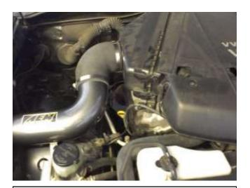
AEM® intake system installed
