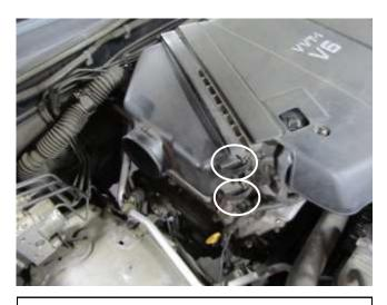
c. Attach the clips that were undone in step 2d.
