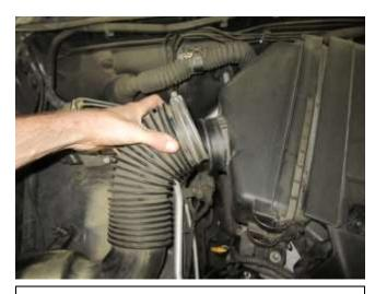
b. Detach the intake tube from the air box.
