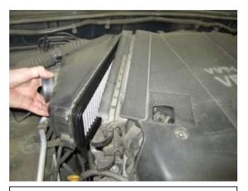
b. Re-install the AEM filter and air box lid to the air box base. Make sure that the back of the lid is correctly hinged.
