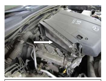
f. The hydrocarbon trap filter will remain in the air box; do not attempt to remove it. The hydrocarbon trap filter is an emission control device and should not be removed to retain legal status in California
