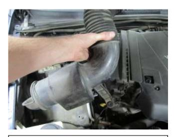
c. Pull the intake tube out of the fender and remove from the vehicle. **NOTE:** Do not discard your factory intake components.
