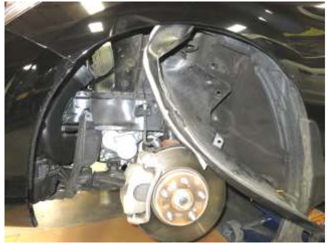
k. Once the fender liner is free, it can fold neatly back behind the brake assembly as shown.
