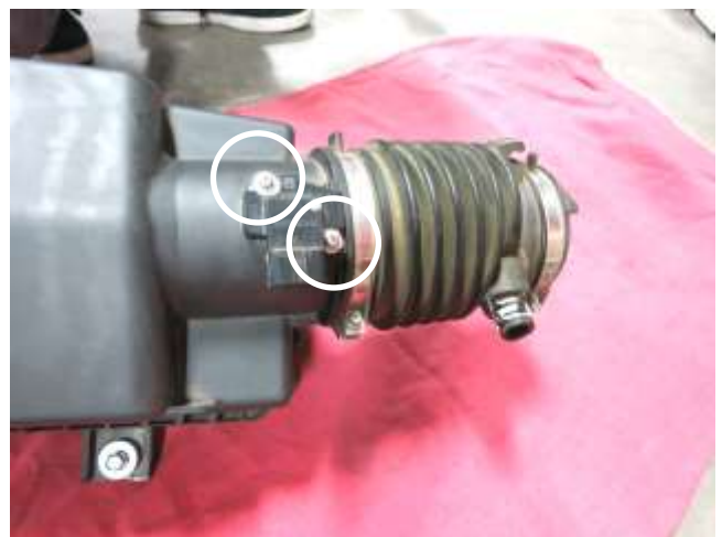
n. Remove the two screws securing the MAF to the stock air box. These will be reused in step 3c.
