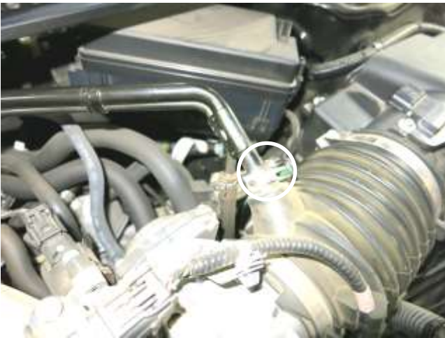
c. Squeeze the spring clamp and remove the vent line from the stock intake tube. This will be reused in step 3f.
