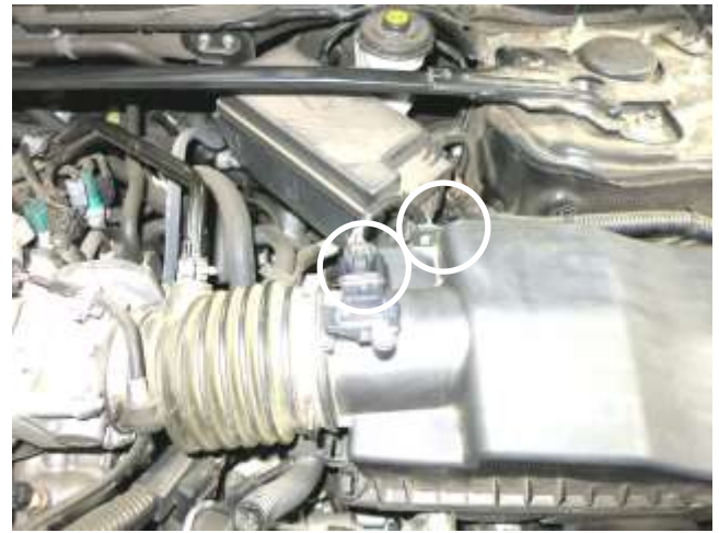
b. Depress the MAF electrical connector and squeeze the green clip to remove the wiring harness from the stock air box.
