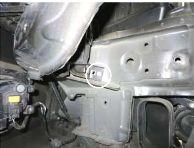
m. Remove the bolt securing the above bracket . This bolt will not be reused.
