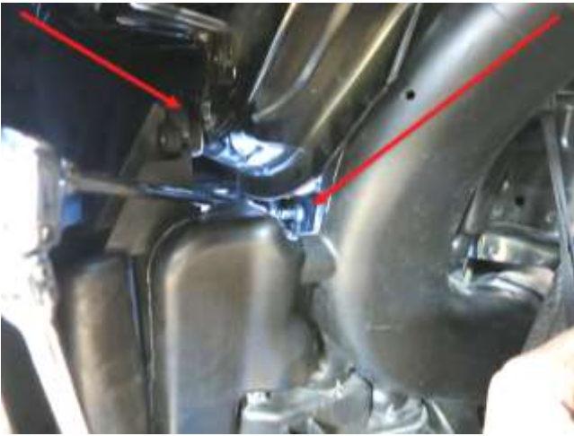
l. First remove the bolt shown above on the left, allowing you to lower the resonator. Using a short 10mm socket and u-joint on the end of at least 14" of extension
