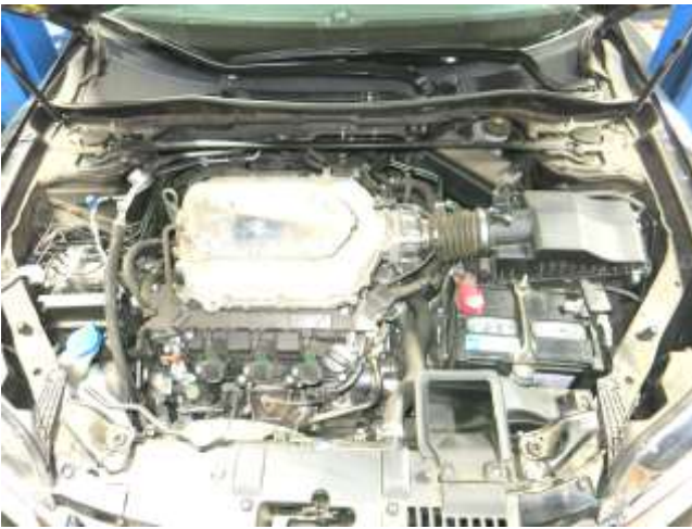
a. Remove the engine cover by lifting straight up.
