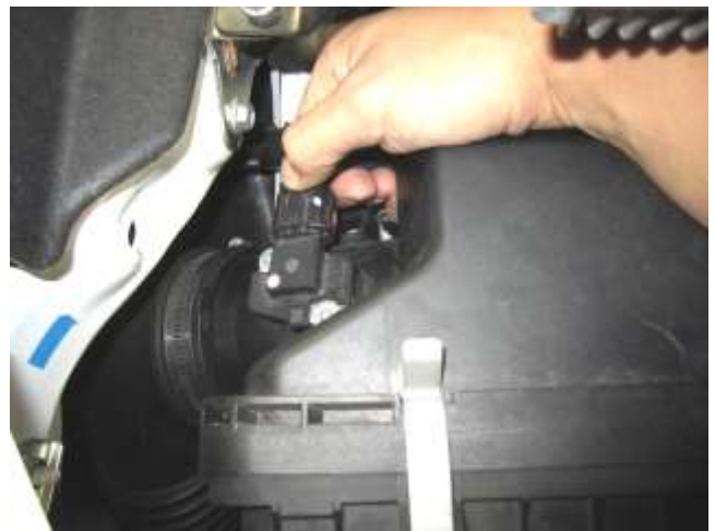
b. Depress the tab on the mass air flow sensor plug and disconnect it from the MAF sensor.
