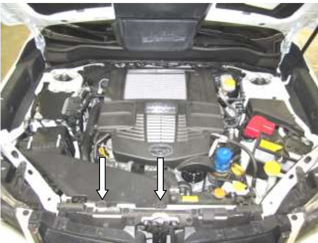
a. Remove the two plastic clips and the factory fresh air inlet duct.
