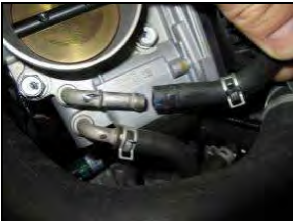
Y. Place a rag under the hose to catch any spilled coolant. Release the clip on the throttle body coolant hose and pull the hose off.
