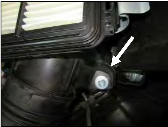
G. Remove the M6 bolt holding the air box in place.
