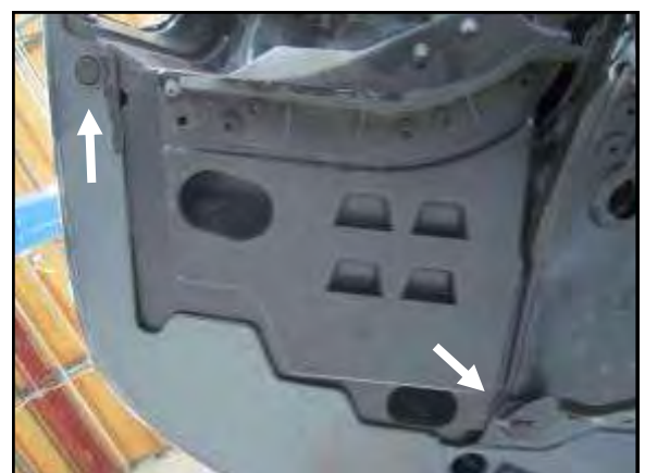
P. Remove the two bottom clips holding the splash shield.
