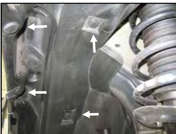
O. Remove the four front upper clips securing the splash shield.
