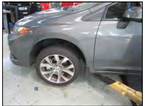
J. Raise the front of the vehicle with a jack. Support your vehicle using properly rated jack stands before wheel removal or while working under the vehicle.
