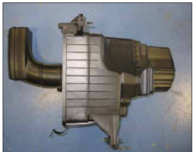
j. Remove the lower air filter housing and bypass pipe assembly from the engine compartment.
