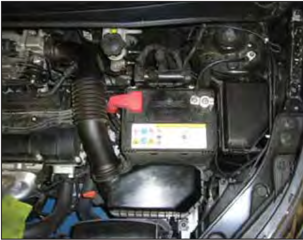
Factory airbox system installed
