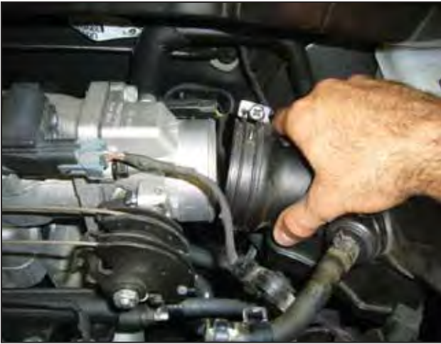
e. Loosen the large hose clamp and disconnect the air intake tube at the throttle body.
