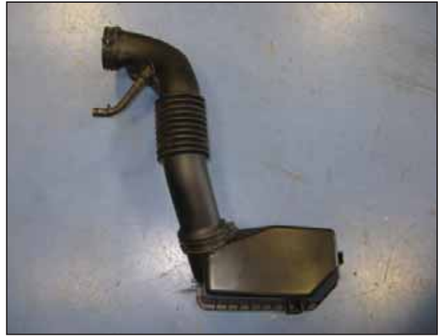
f. Remove the factory air filter housing lid and air intake tube from the engine compartment.
