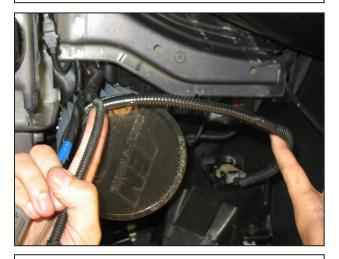
h. Wrap the supplied convoluted slit over the exposed fog light wires and secure with electrical tape. Unclip the washer fluid hose from the clip that attaches it to the inner fender. Push the hose and the two wire connectors up top behind the headlight.
