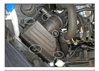
b. Loosen the hose clamp on the inlet hose. Unclip the four clips on the air box top and remove it from the vehicle.
