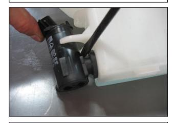
k. Pry the washer pump out of the grommet and set it aside. Also remove the grommet and set it aside.
