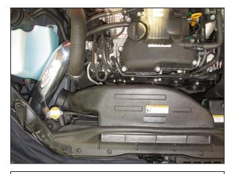
t. Check the fitment of the intake system and ensure there is clearance between the inlet pipe and its surrounding components. Once proper fitment is achieved, tighten all hose clamps and the M6 nut on the rubber mount. If desired, reinstall the stock air scoop removed in step 2a.
