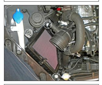
c. Remove the three M6 bolts securing the lower air box, then remove the lower air box.
