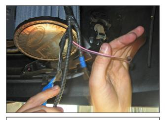
g. If the vehicle is equipped with fog lights, unwrap the convoluted slit to expose the wires, then remove the fog light wires.
