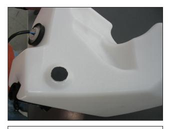
q. Stick the self-adhesive rubber pad onto the small bump that protrudes from the washer bottle.
