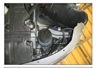
f. From underneath the vehicle, install the air filter with the #9460 hose clamp. Slide the air filter onto the end of the inlet pipe until the pipe reaches the stop inside the filter. Once proper fitment is achieved, tighten the hose clamp.
