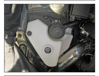
r. Lower the washer bottle assembly into place as shown. Plug the washer hose and wire harness connector to the pump. Plug in the level sensor connector and tuck the wires away. Secure the washer bottle into place with the two M6 bolts removed in step 2h.
