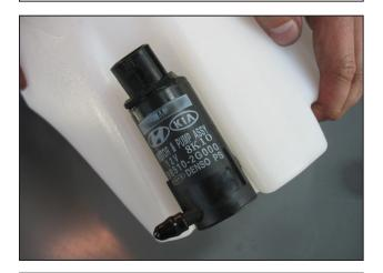
n. Apply some liquid soap solution to the washer pump and insert it into the grommet. Firmly press the pump all the way into the grommet.
