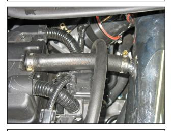
I. Install the 5/8" hose onto the upper intake pipe nipple and the valve cover nipple. Secure each end with a 1 1/16" hose clamp.
