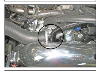
s. Insert the tree-push mount zip tie into the bracket of the upper intake pipe bracket. Secure the MAF sensor harness as shown and trim the excess zip tie. Plug the MAF harness connector into the MAF sensor.
