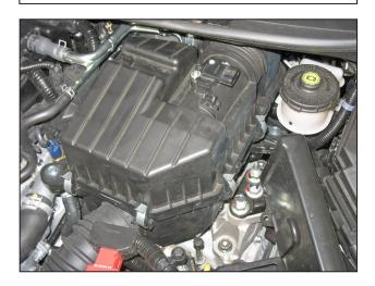
d. Unclip the metal clips securing the air box lid to the lower air box.
