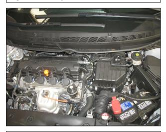
Stock air box system installed
