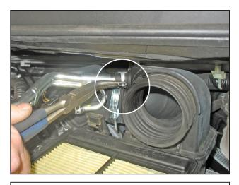
f. Disconnect the PCV hard line from the rubber inlet.
