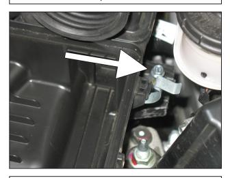
j. Remove the second bolt securing the stock air box to the vehicle.
