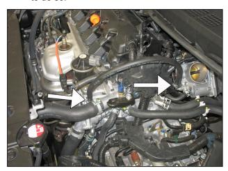
b. Use the supplied 3/8" hose to replace the coolant line removed in steps 2m and 2n and secure it using the 2 supplied hose clamps.
