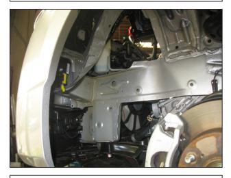
u. Remove the resonator assembly from the vehicle.
