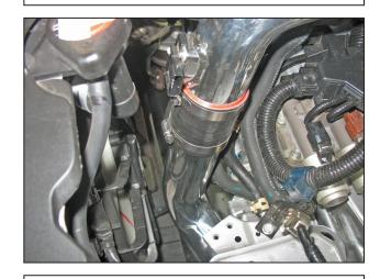
o. Align the lower intake pipe with the upper intake pipe and orient as shown. Insert the lower intake pipe into the upper intake pipe's coupler and loosely secure the #9440 hose clamp.
