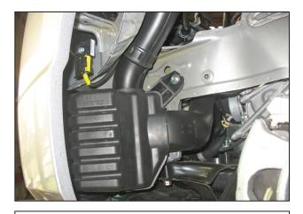
t. Remove the two bolts securing the lower resonator to the vehicle.
