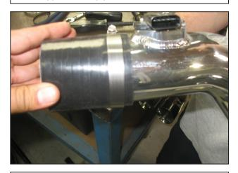
g. Install the 2.50" X 3.00" silicone hose onto the upper intake pipe as shown.
