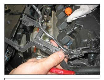
q. Remove the hard plastic casing on the MAF sensor harness to expose the wires.
