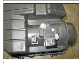
v. Remove the mass air flow (MAF) sensor from the lid of the stock air box.
