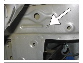
m. Install the second rubber mount in the threaded hole exposed in step 2u.
