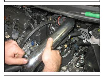
h. Insert the upper intake pipe into the silicone hose installed on the throttle body.
