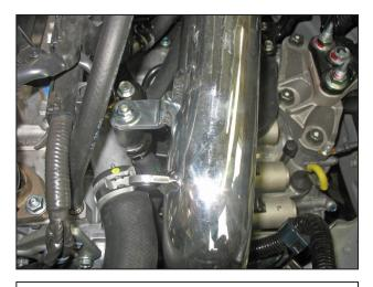
k. Install the washer and serrated nut on the rubber mount to sandwich the bracket.
