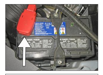
o. Disconnect the positive terminal and loosen the two nuts securing the battery tie down. Remove the battery tie down and the battery.
