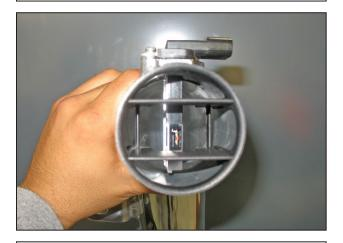
f. Install the supplied air flow straightener and orient as shown. The fins should be perpendicular to the MAF sensor.
