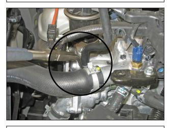
n. Remove the other side of the coolant line connected to the engine.
