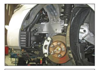
s. Remove all the clips securing the fender liner to the front of the vehicle and move it out of the way as shown.
