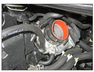
c. Install the  $2.50^\circ$  X  $2.00^\circ$  silicone hose on the throttle body and loosely secure two #9440 hose clamps.
