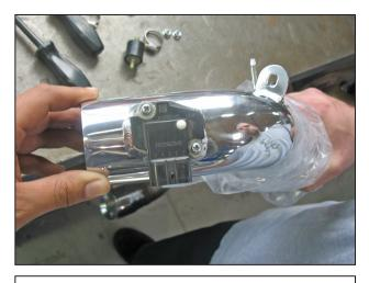
e. Using the stock bolts, secure the MAF sensor to the upper intake pipe.
