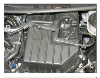
c. Remove the wire harness from the clips located on the air box lid.
