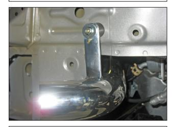
n. Install the lower intake pipe aligning the bracket with the installed rubber mount. Loosely secure the bracket with a supplied washer and serrated nut.
