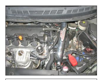
AEM® intake system installed
