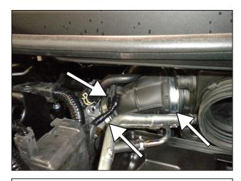
k. Loosen the hose clamp securing the stock inlet tube to the throttle body and air box. Also remove the wire harness from the inlet tube.
