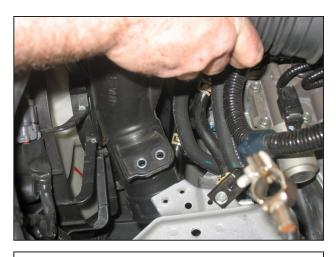
p. Remove the two bolts securing the lower inlet tube to the vehicle.
