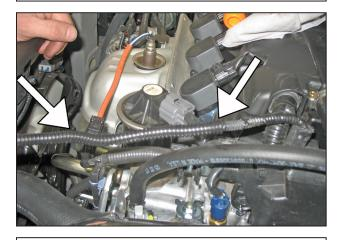
r. Use the supplied convoluted slit loom to cover the wires that were exposed in the previous step.
