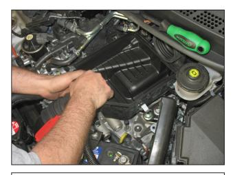
I. Disconnect the rubber inlet duct from the front of the air box, then remove the air box from the vehicle. Remove the inlet tube from the throttle body.
