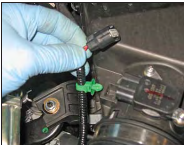
c. Disconnect the mass airflow (MAF) sensor from the vehicle.
