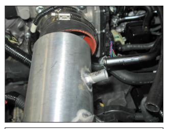
h. Insert the upper intake pipe (2-6831) into the previously installed reducer coupler on the throttle body. The end of the intake pipe closest to the PCV nipple and MAF adapter should install into the throttle body coupler. Secure in place with a hose clamp (9452).
