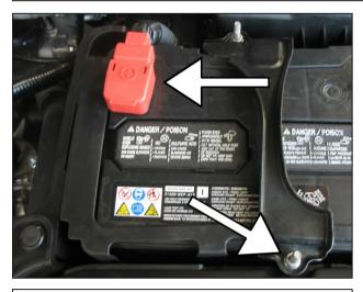
f. Remove the battery by removing the battery tie down and disconnecting the positive terminal.
