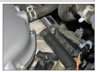
d. Insert the  $\frac{1}{2}$ " hose (5-5016) onto the crank case, securing with the 1" hose clamp. Leave the other end open for now.
