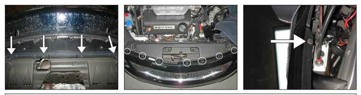
v. Remove the front bumper by removing the side and bottom clips as indicated. Please do not forget to remove the Phillips screw (picture on the far right) from both the left and right side of the vehicle. If the vehicle is equipped with fog lights, unplug them before removing the bumper.
