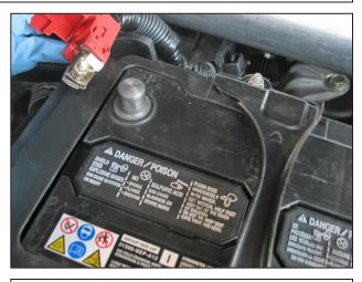
s. Install the battery and reconnect the positive lead.
