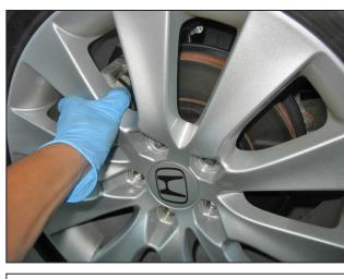
u. Install the driver side wheel using the factory torque specification (see owner's manual).
