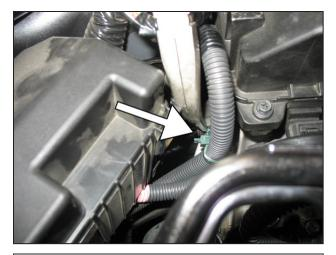
j. Remove the retaining clip indicated in the picture.
