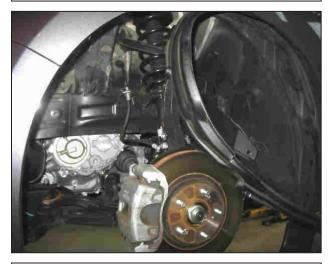
r. Push back the fender liner as shown in the picture.
