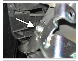
w. Locate and remove the 10mm bolt holding the remainder of the air box system to the chassis. Automatic Transmission Vehicles: Please proceed to step 2x.
