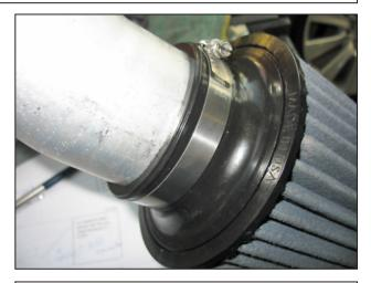
n. Install the air filter element onto the non-bracket side of the lower intake pipe (2-6832). Secure in place with the provided hose clamp (9456).
