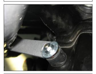
i. Slide the upper intake pipe's bracket onto the previously installed rubber mount; loosely secure with a 6mm washer and nut.
