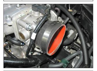
e. Place the reducer coupler (5-323) onto the throttle body with the smaller side over the throttle body. Secure the smaller side of the coupler with the provided hose clamp (9444).
