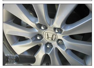
o. Raise the front of the vehicle with a jack. Refer to your owner's manual for proper jack and jack stand placement to properly support vehicle. Support your vehicle using properly rated jack stands before wheel removal or while working under the vehicle. **NEVER WORK UNDER A VEHICLE WITHOUT USING JACK STANDS.** Remove the driver-side front wheel with a 19mm socket.
