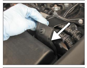
m. Push the air box panel unit out from the dowel and set aside.
