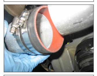
o. Connect the lower intake pipe to the upper intake pipe with the straight coupler (5-326) and a (9452) hose clamp.
