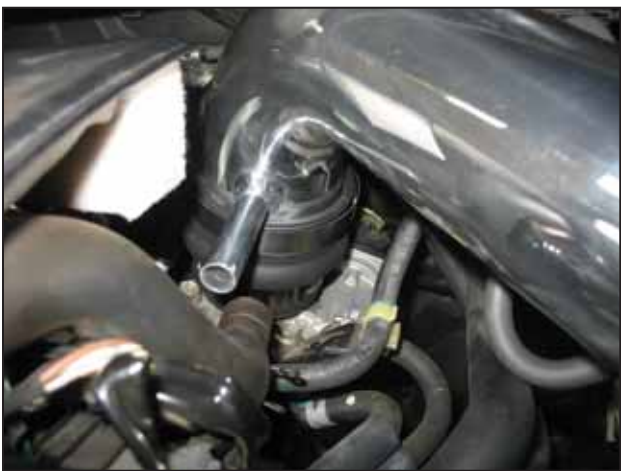
j. Install the upper intake pipe into the hump hose connected to the throttle body.
