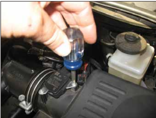
c. Remove the MAF sensor from the air box assembly. The MAF sensor will be reinstalled with the AEM® intake system.
