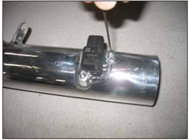
g. Install the MAF sensor into the upper intake pipe using supplied bolts (1-2051).
