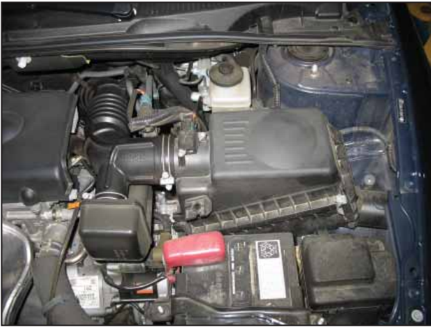
Factory air box system installed
