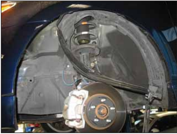
r. Pull the driver side fender liner away from front fender and secure it behind the front brake rotor.
