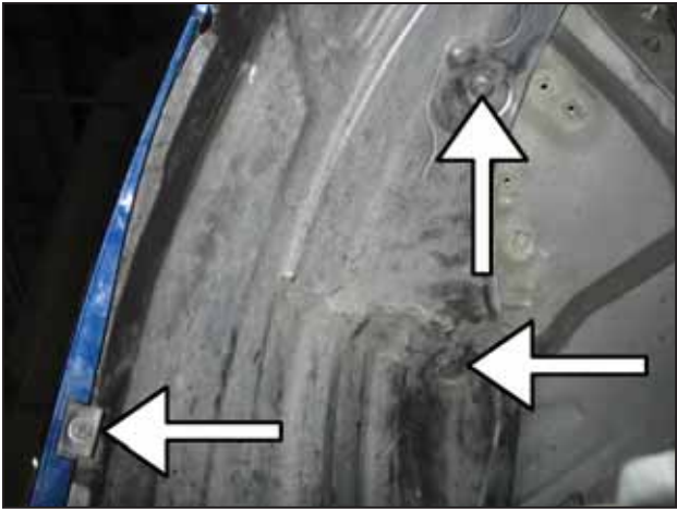
q. Remove the screw and clips securing the driver side fender liner.
