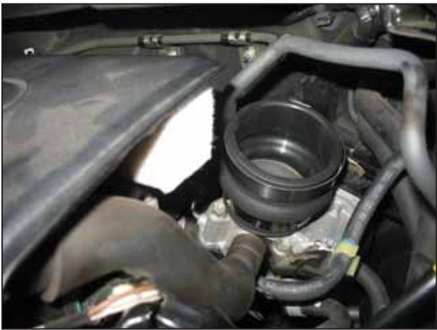
h. Install the small end of the hump hose (5-574) onto the throttle body and secure with #40 hose clamp. Install a #48 hose clamp loosely over the large end of the hump hose.
