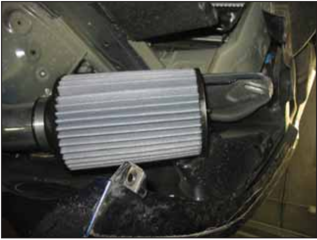
f. Attach the air filter to the lower intake pipe and secure with #52 hose clamp.
