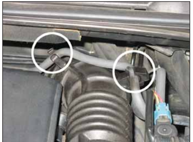
d. Unclip VSV hose from intake tube.
