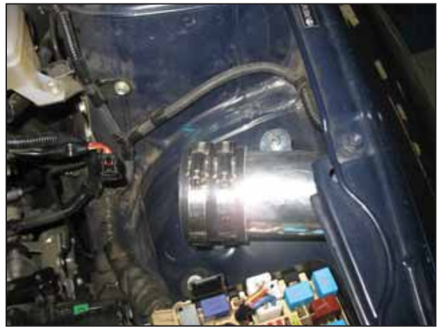
i. Slide the coupler (5-302) and two #48 hose clamps over the lower intake pipe.
