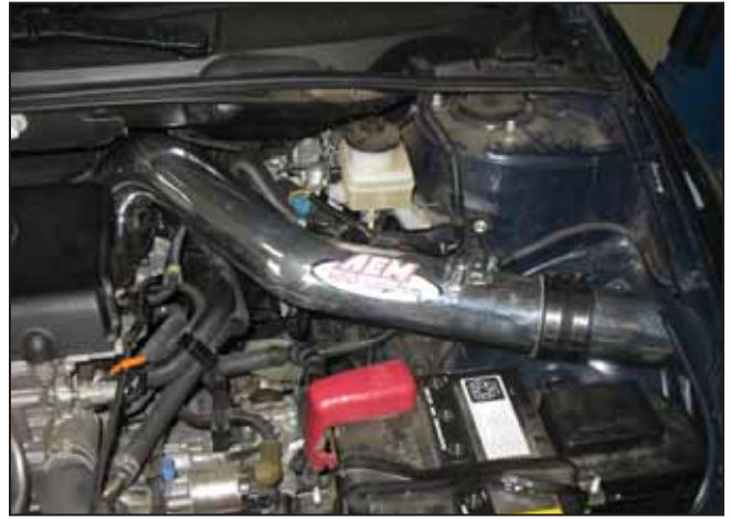
AEM® intake system installed
