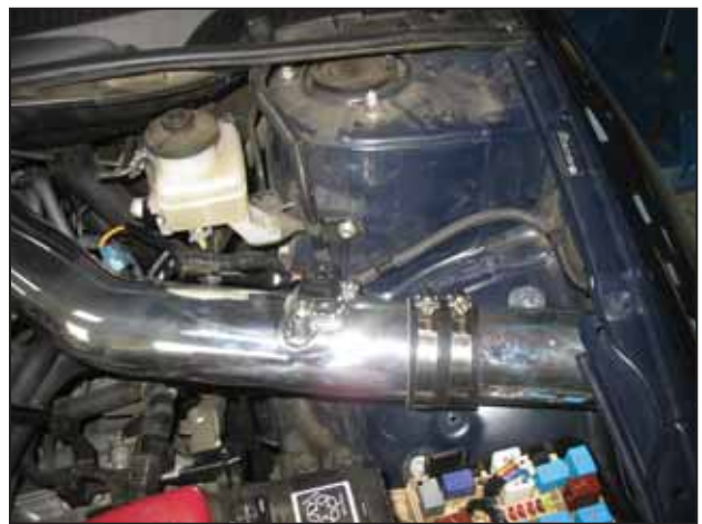
k. Align the upper intake pipe with the lower intake pipe and slide the coupler over the upper pipe so that the coupler covers both tubes evenly. Loosely secure the #48 hose clamps.
