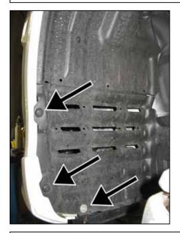
m. Remove the driver side fender well liner, it is secured to the wheel well with plastic clips and a 10mm hex bolt.
