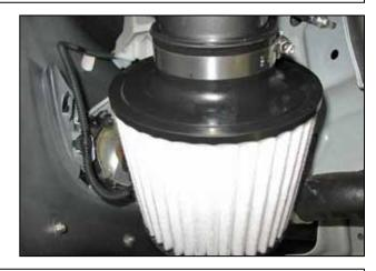
u. Install the air filter (21-2027DK) onto the lower end of the lower intake pipe (2-6792). Secure the air filter onto the intake pipe with a provided #44 hose clamp.
