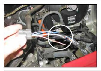
d. Locate the MAF sensor wire harness connector, measure 2 inches from the back of the connector and cut the four wires.
