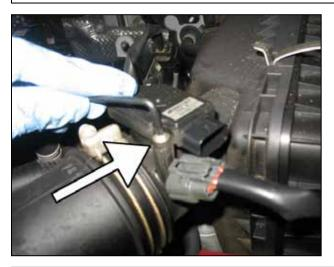
g. Remove the MAF sensor with the provided T20 L-key.
