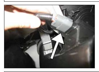
t. Plug the MAF sensor connector into the MAF sensor.
