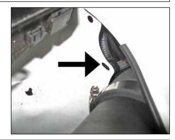
j. Remove the side harness clip by pushing it out.
