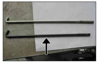
c. Replace the factory j-hook with the shorter j-hook that is supplied with installation kit.
