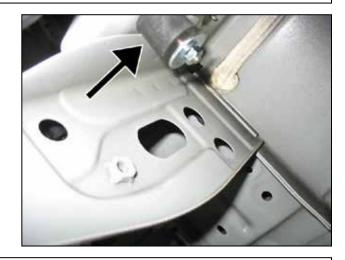
q. Install the rubber mount in the indicated hole, secure in place with a 6mm fender washer and 6mm serrated nut. Attach a 6mm fender washer and 6mm serrated nut to the stud on the bottom side of the rubber mount.
