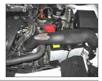
AEM<sup>®</sup> intake system installed
