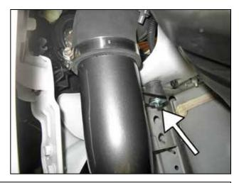
s. Feed the lower intake pipe through the bottom side of the fender well. Align the intake pipe's bracket onto the rubber mount and loosely secure in place with the provided 6mm washer and the 6mm nut.
