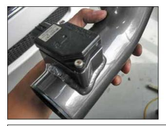
r. Install the MAF sensor into the lower intake pipe (#2-6792) with the provided hardware fasteners (#1-2023).
