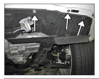
k. Raise the front of the vehicle with a jack. Refer to your owner's manual for proper jack and jack stand placement to properly support vehicle. Support your vehicle using properly rated jack stands before wheel removal or while working under the vehicle. **NEVER WORK UNDER A VEHICLE WITHOUT US-**
