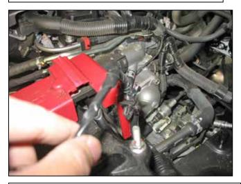
j. Wrap the remaining section of the wire harness with electrical tape.
