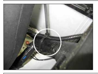
v. Secure the MAF sensor wire harness in place with a zip tie as shown.
