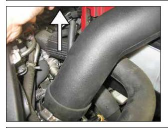
p. Insert the upper intake tube (9-6791) into the throttle body coupler. Position the intake tube so the nipple is pointing upward as shown. Use a provided hose clamp to loosly secure in place.
