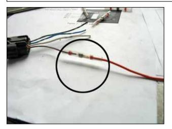
f. Using the schematic on page 3, use the provided connectors to extend each wire.
