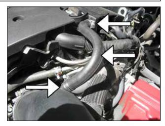
w. Attach the provided PCV hose onto the crankcase inlet and intake pipe nipple. Secure each end with a provided hose clamp.
