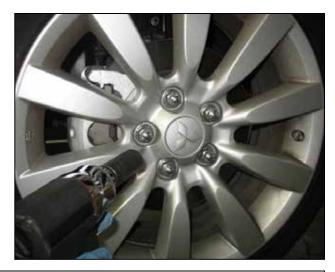
I. Remove the front drivers side wheel with a 21mm socket.
