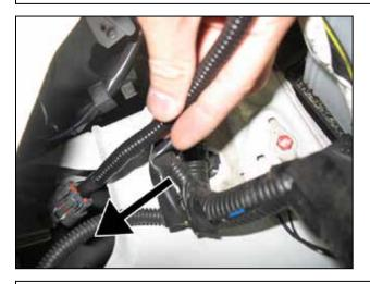
I. Route the MAF sensor harness down into the wheel well area.
