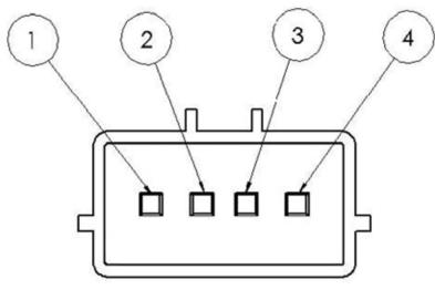
NOTE: PIN 4 on the female MAF sensor plug corresponds to the flow of the MAF sensor. Figure 1 ~ MAF Sensor Plug (Harness Side)
