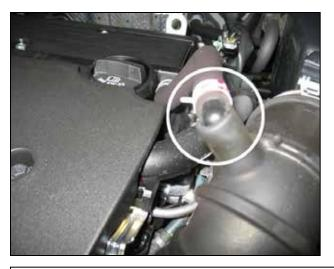
c. Remove the PCV tube from the crankcase side.
