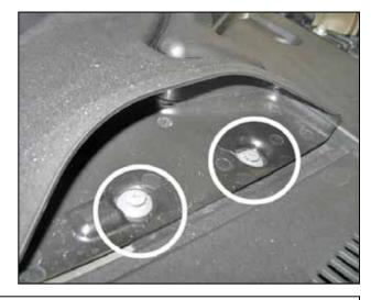
b. Remove the front section of the stock air duct, there are two Philips head screws securing it in place.
