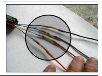
g. Mount the wire ends into each connector as shown. Once the wires are properly positioned within each connector, use a heat gun to apply heat so the solder/insulation melts and secures the wires in place. Repeat this step for the remaining 3 wires.
