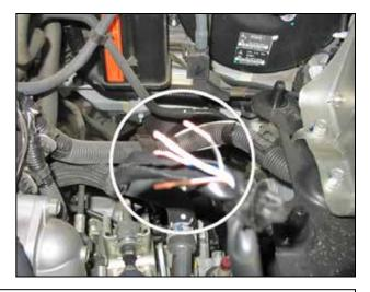
i. Locate the wires on the vehicle side of the harness. Attach the extended harness to the vehicle side harness using the same process used to extend the wire harness in step 3g.
