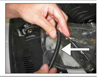
k. Sheath the wire harness with the convoluted slit and secure each end with electrical tape.
