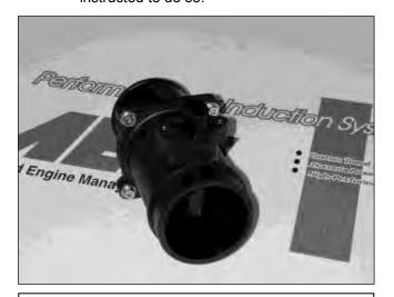
b. Bolt the adaptor to the MAF sensor using the factory bolts.
