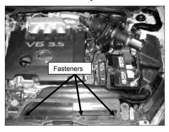
a. Remove the three plastic fasteners that secure the air scoop and remove it.
