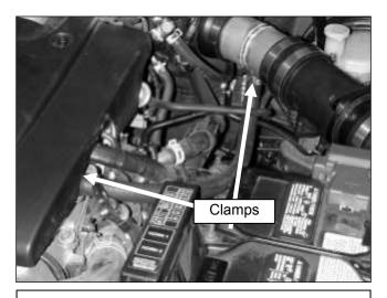
h. Install the included 5/6" breather hose onto the cam cover vent and the nipple on the upper pipe, using the supplied 1" hose clamps.
