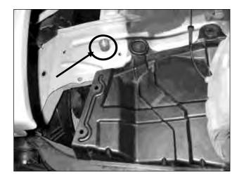
e. Install the supplied rubber isolator on the inner fender, as shown.
