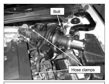
b. Remove the bolt securing the connector tube to the chassis, loosen the hose clamps as shown, and remove the connector tube assembly.
