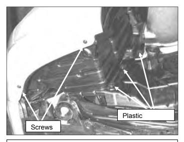
e. Remove the three plastic fasteners and two screws securing the inner fender liner. Remove the fender liner to gain access to the inner front bumper.
