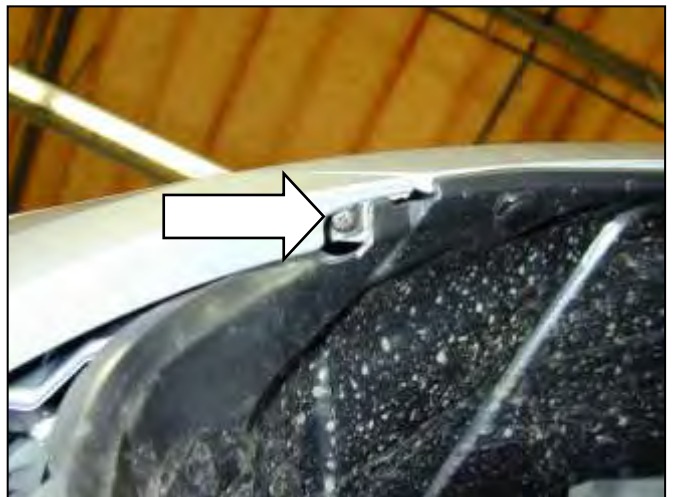
l. Remove the screw holding the corner of the front bumper cover.
