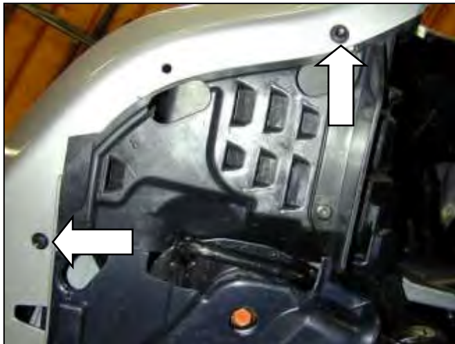
i. From underneath the vehicle, remove the fasteners shown in the picture.
