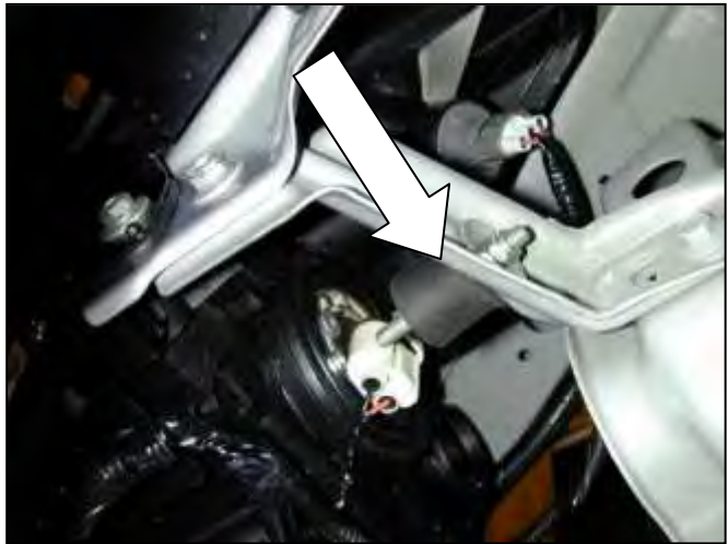
c. Install the rubber mount in the bracket behind the front left headlight as shown in the picture. Secure it in place with a washer and Nylock nut as shown.
