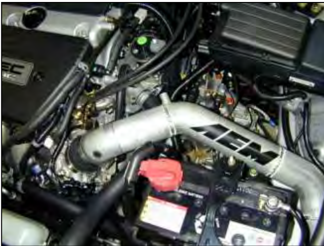
d. Insert the AEM® intake pipe into the engine bay. Line up the bracket of the intake pipe with the rubber mount while also inserting the intake pipe into the coupler on the throttle body.
