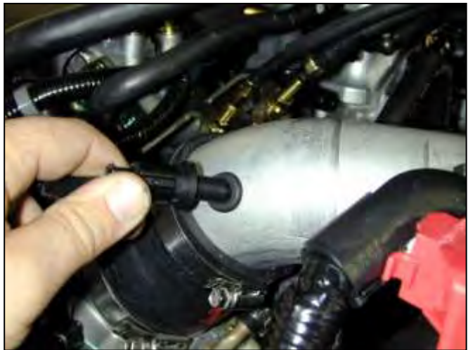
e. Install the included rubber grommet into the small hole on the intake pipe. Insert the IAT sensor into the hole.
