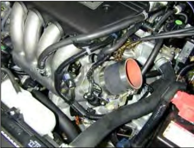
b. Place the coupler on to the throttle body. Install a #44 hose clamp around the throttle body and a #40 on the other end. Do not tighten the hose clamps.
