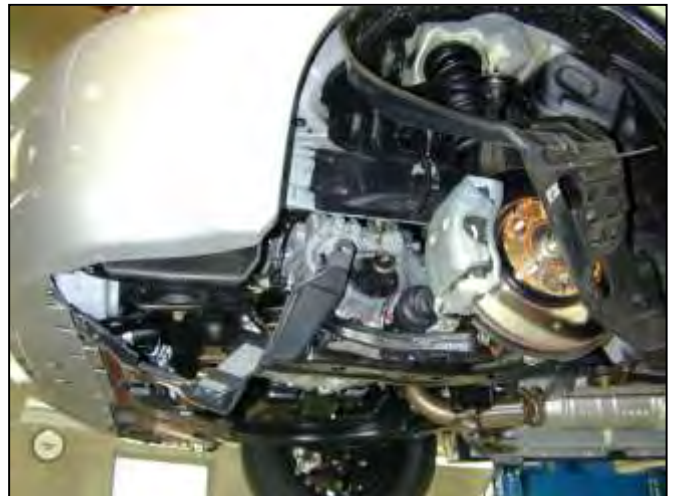
j. Tuck the fender liner out of the way behind the brake rotor.
