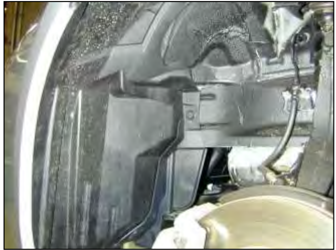
h. Remove the fasteners securing the driver-side wheel well liner.
