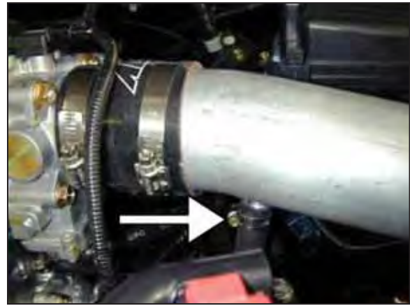
k. Attach the opposite end of the breather hose onto the nipple of the intake pipe. Secure it with a supplied 1" hose clamp.
