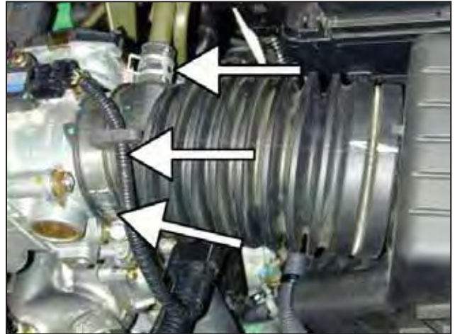
b. Remove the inlet tube by removing the hose clamp, the spring clamp and releasing the wire loom from the inlet tube's clip. Pull the breather hose off the inlet tube, then remove the inlet tube.
