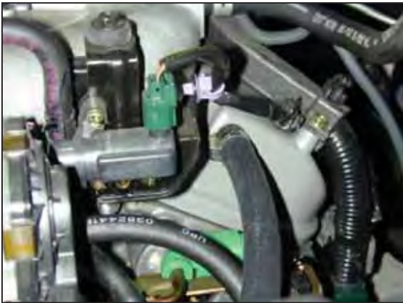
j. Install 1/2" ID hose over the breather nipple on valve cover. Secure it with a supplied 1" hose clamp.
