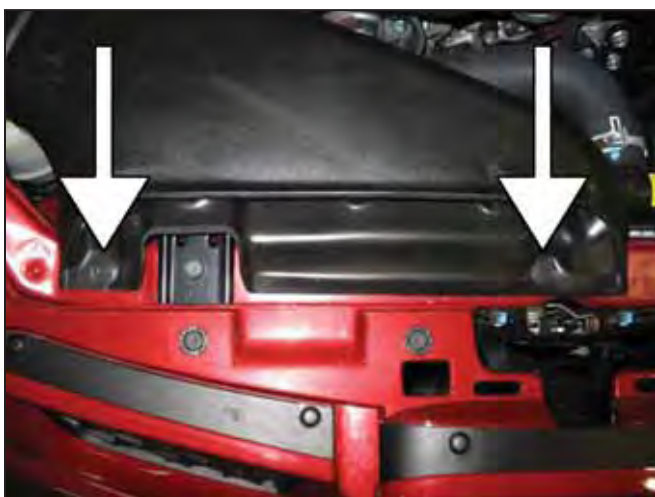
c. Remove the two mounting bolts holding the air inlet scoop and remove the scoop from the vehicle.
