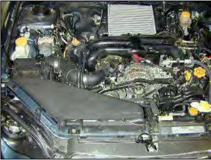
c. Remove two bolts to the air box air duct. Remove air duct.
