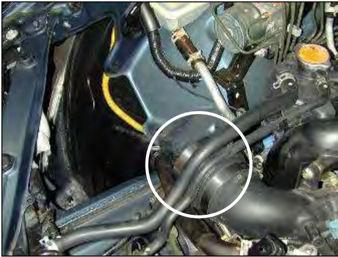
b. Attach 2.75" hump hose to the plastic turbo inlet. Attach hose clamps but do not tighten.
