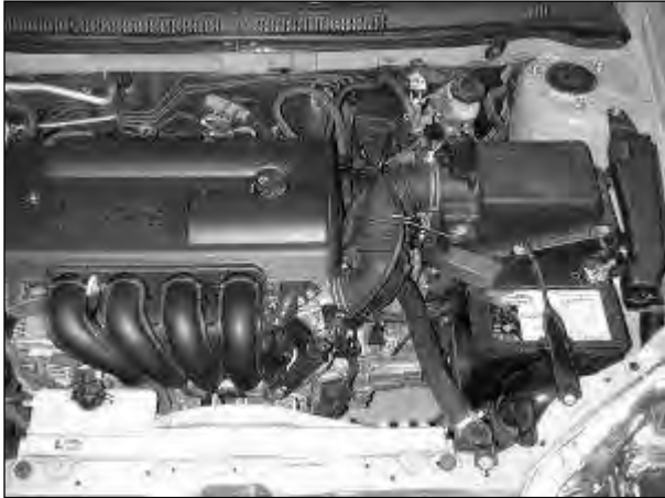
Factory air box system installed
