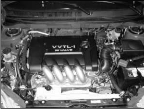
Factory air box system installed
