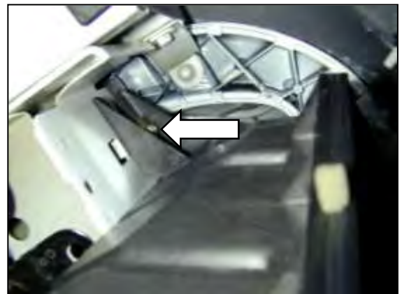
j. Remove the screw in the upper front section of the lower airbox. Remove the lower airbox.
