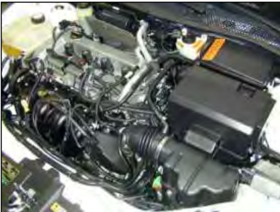
a. Factory airbox system installed.
