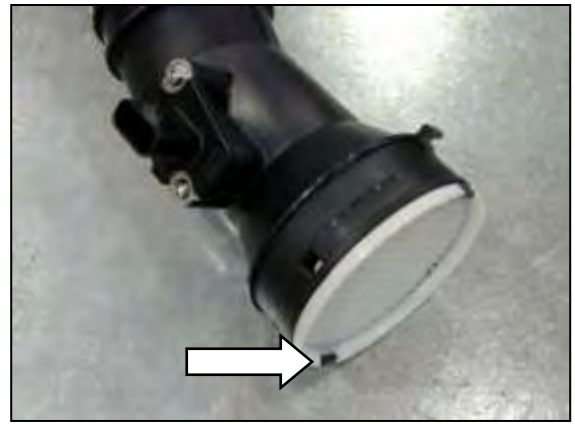
f. Remove the MAF sensor housing and confirm that the air straightener is still attached to the lower opening.
