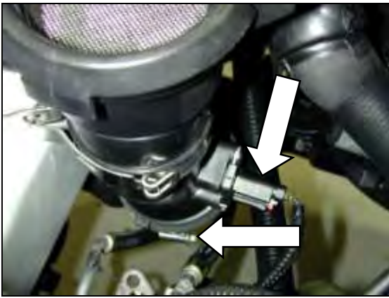
e. Unplug the MAF sensor. Loosen the hose clamp at the bottom of the MAF housing.
