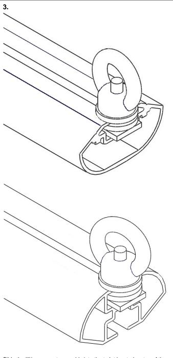
Slide the lifting eye nut assembly into the t-slot located on top of the load bar.
