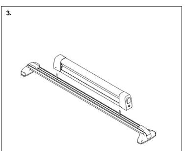
Position the two carriage bolts so that the bolts line up with the holes on the bottom of the ski carrier. Set the ski carrier down on the carriage
