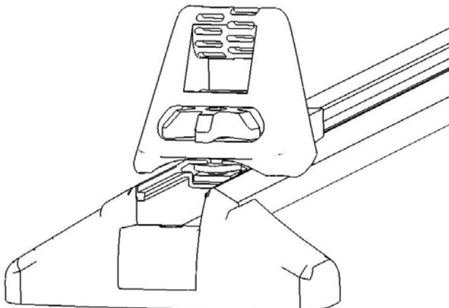
Align the tab on the front of the load stop so that it slides into the channel. Loosen the daisy dial on the load stop so that the nylon washer rests inside the channel on the crossbar.
