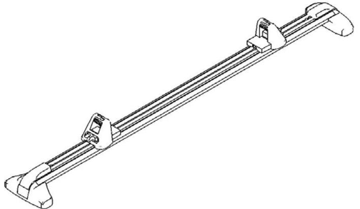
Slide two load stops into the crossbar. The load stops should be orientated such that they face each other. Replace end cap after load stops are in place.
