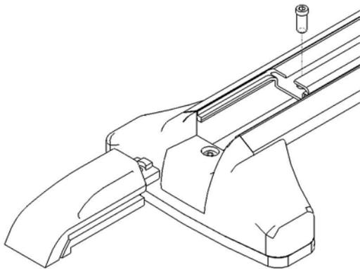
Remove the end cap from the crossbar bar by loosening the narrow shoulder hex screw.
