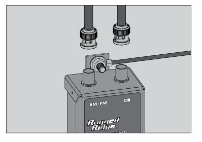
11. Connect JK Radio Cable to factory antenna cable.
