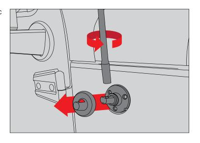
2. Remove three screws from antenna base and unplug factory antenna cable. Save screws for later use.
