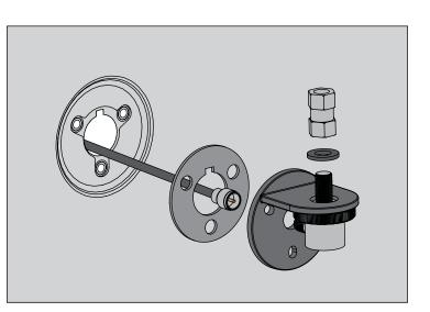
6. Using screws removed in step 2, install Antenna Mount on fender.
