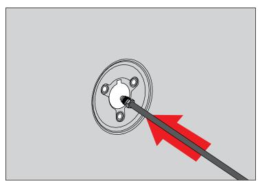
5. Install Antenna Stud on Antenna Mount. Insert Antenna Cable through Antenna Mount and Gasket and connect to Antenna Stud.
