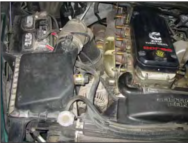
Factory airbox system installed
