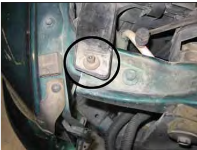
c. Remove the nut securing the front of the air filter housing to the chassis. Lift up on the air filter housing and remove it from the engine bay.
