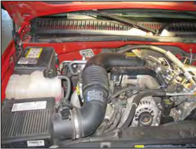
Factory air box system installed
