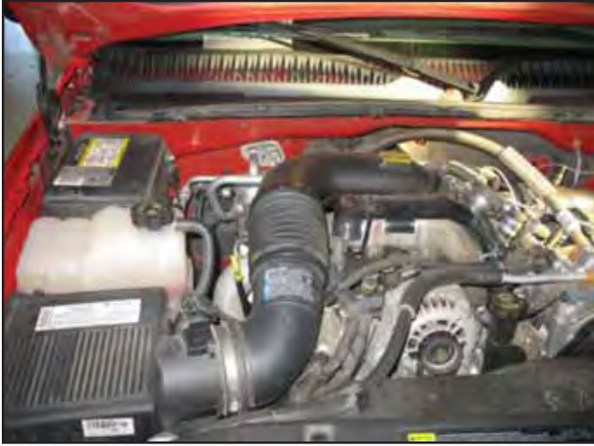
a. Factory air box system installed.
