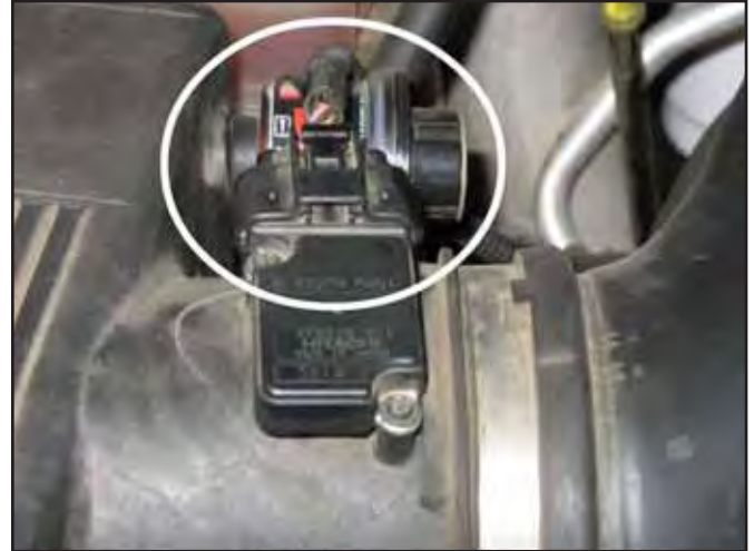
b. Unplug the mass air flow sensor (MAF) wiring harness.
