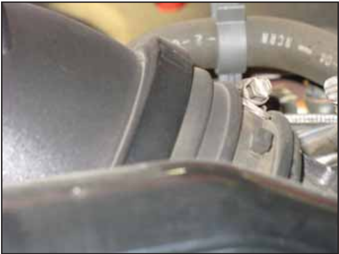
c. Lift up on the intake resonator to pop it off the mount and gain access to the hose clamp on the inlet tube. Loosen the hose clamps on both ends of the inlet tube.
