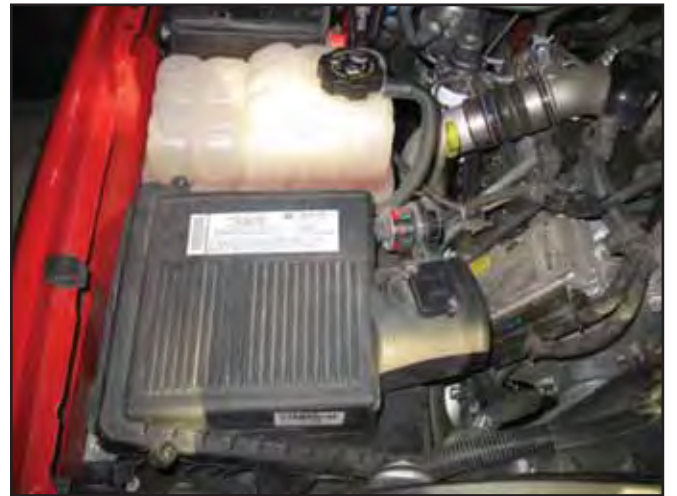
d. Remove the inlet tube and resonator from the engine bay.
