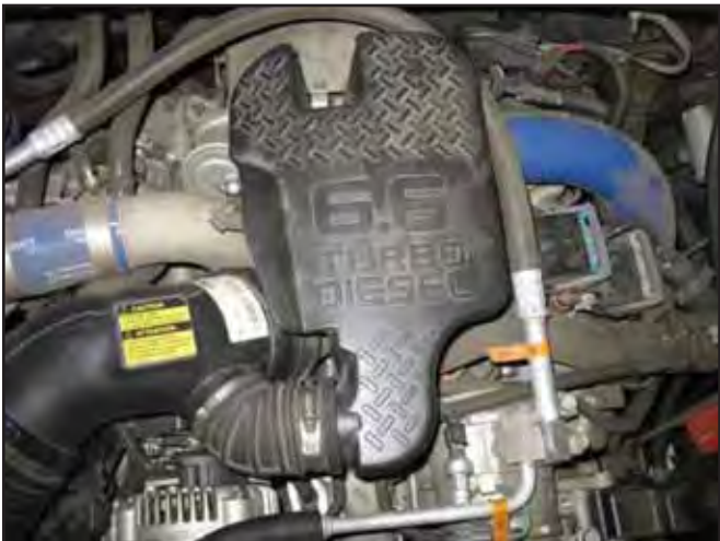
c. Lift up on the intake resonator to pop it off the mount. Loosen the hose clamps on both ends of the inlet tube.
