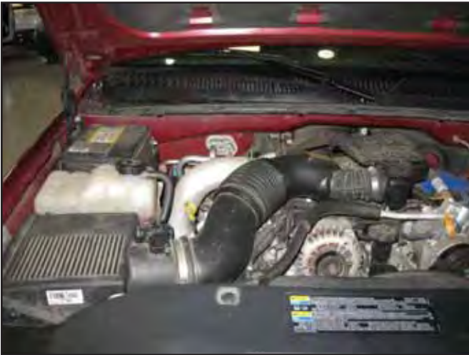
Factory air box system installed
