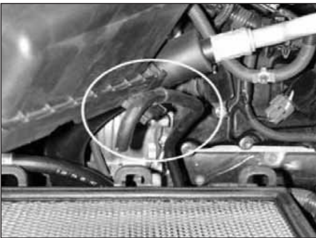
g. Raise the upper airbox. If the truck is equipped with 4WD, disconnect the differential breather hose from the airbox.
