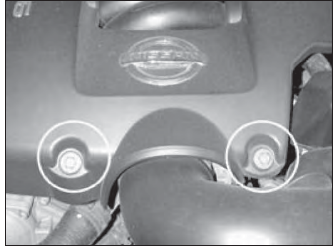
b. Remove the two screws securing the engine cover and remove the cover.
