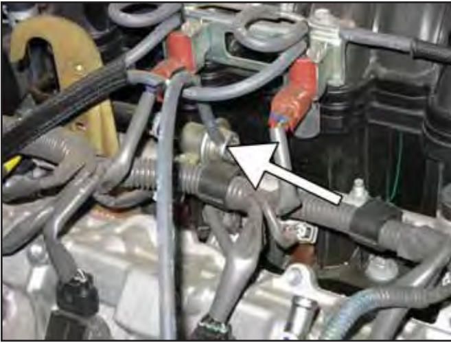
k. Disconnect the opposite end of the 5/32" ID hose disconnected in step 2f.
