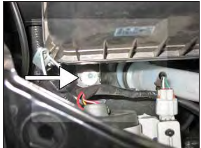
h. The final bolt to remove the stock air box is located behind the passenger side headlight.
