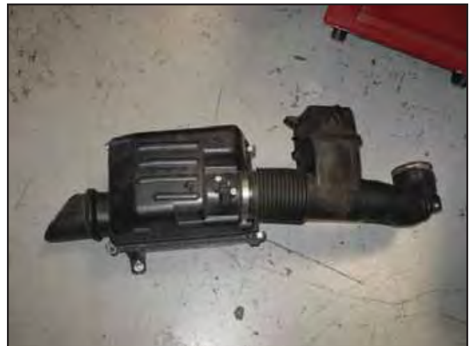
j. After, pulling the intake tube away from the throttle body, the air box and intake tube, should be pulled out as an assembly as shown.
