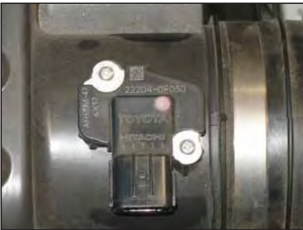
m. Remove the MAF sensor from the stock housing removed in step 2j. Be extra careful with this sensor.
