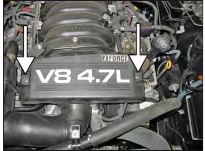
b. Loosen the two bolts securing the engine cover to the engine. Then, remove the engine cover.
