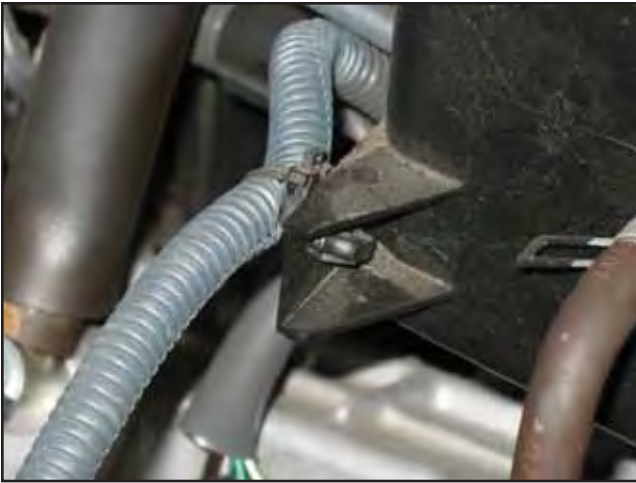
e. Disconnect the stock zip tie that is securing the MAF harness to the air box. Do not cut this zip tie it will be reused later.
