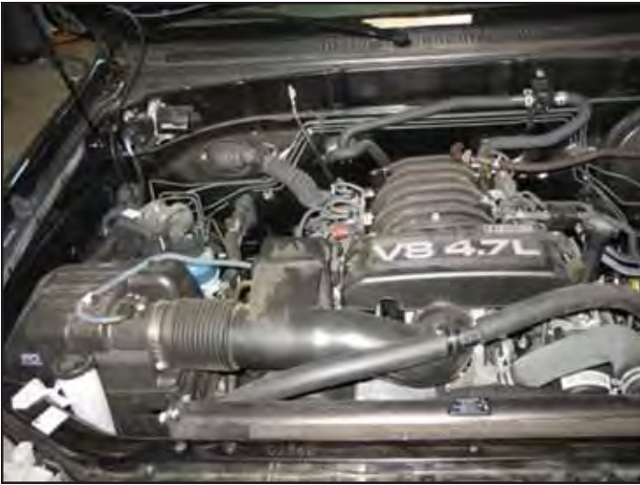
Factory intake system installed
