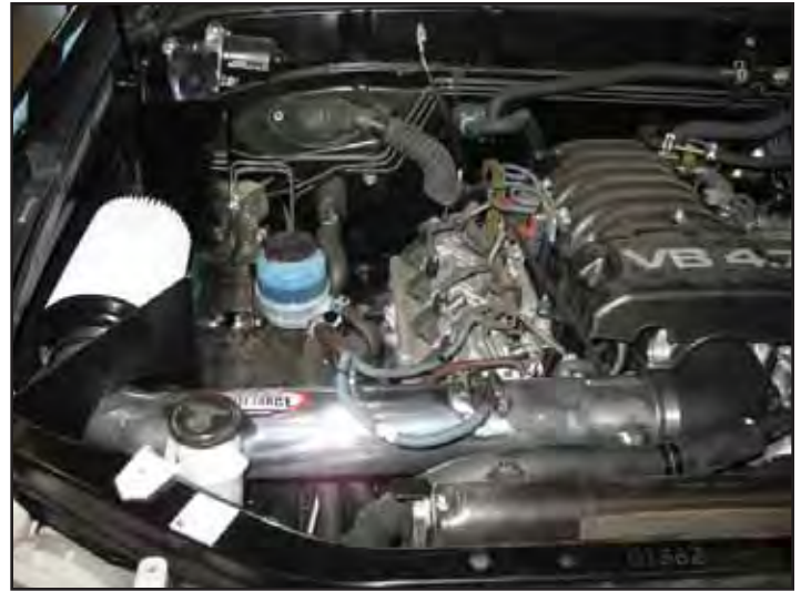
AEM® intake system installed
