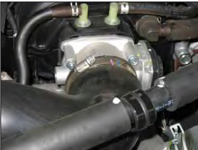
i. Loosen the hose clamp securing the stock intake tube to the throttle body. Gently pull the stock intake tube toward the front of the vehicle.
