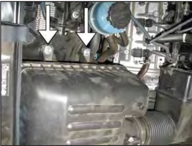
g. Loosen the first two bolts securing the stock air box into the vehicle.
