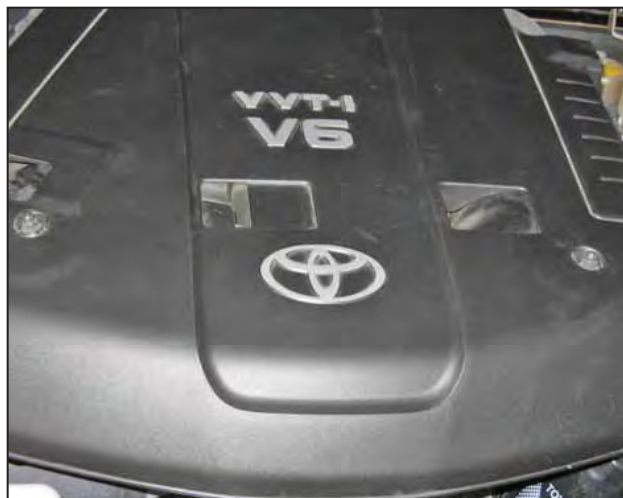
b. Remove the two nuts securing the engine cover.
