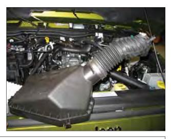
f. Slide the inlet tube off the throttle body and remove the inlet tube and air filter lid as an assembly. Remove the IAT sensor from the inlet tube and set aside in a safe area.
