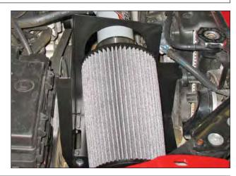
m. Install the AEM® air filter onto the intake tube and secure in place with the supplied #52 hose clamp.
