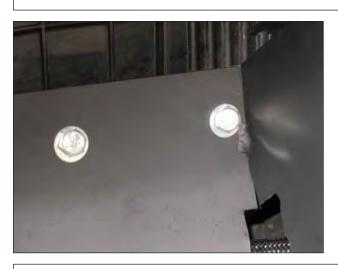
d. Insert the hardware assembled in step 3b through the heat shield holes. Guide the bolts through the spacers that were installed in the previous step.
