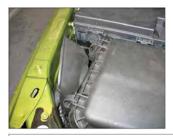
e. Unclasp the two clips securing the airbox lid.
