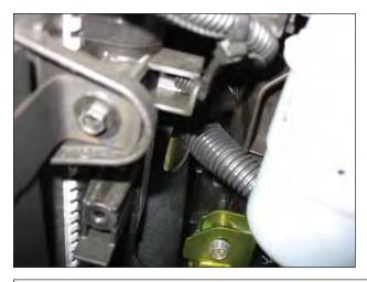
f. Secure the heat shield's tab to the fan shroud using the stock screw removed in step 2i.
