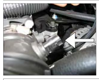
c. Locate the IAT sensor on the inlet tube amd release the wire harness connector from the IAT sensor.
