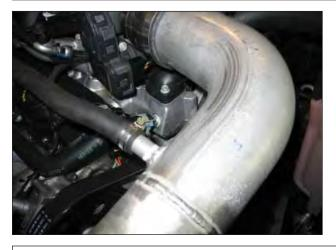
I. Attach the stock breather hose to the intake pipe nipple, secure with the supplied hose clamp.
