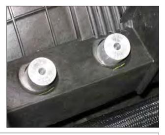
c. Place the two supplied spacers into the inserts that the lower stock grommets were removed from during step 2h.
