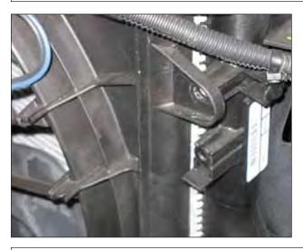
i. Remove the self tapping screw securing the fan shroud. Keep this screw for later use.
