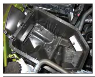
g. Remove the stock air filter and remove the lower airbox by pulling straight up.
