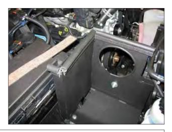
g. Secure the rubber mount to the heat shield with the supplied washer and nut. Install the edge trim onto the heat shield's top edge, also line the heat shield's opening with the supplied rubber edge trim.
