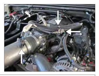
k. Install the grommet into the intake pipe's small inlet hole, then insert the IAT sensor into the grommet. Connect the IAT extension harness to the factory IAT harness and then connect the extension harness connector to the IAT sensor. Secure the wire harness with the supplied zip tie so it is situated in a safe position as shown.
