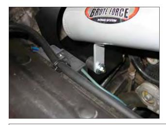
j. Align the intake pipe's bracket to the rubber mount installed on the heat shield and loosely secure the bracket to the rubber mount as shown.
