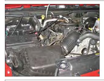
Factory airbox system installed
