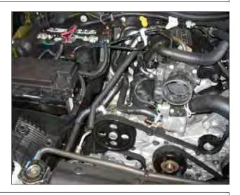
j. Engine bay after the stock airbox system has been removed.
