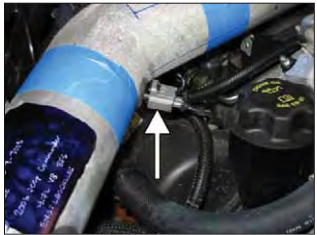
p. Insert the IAT and connector as shown.
