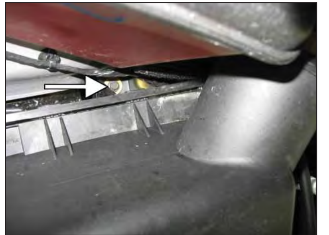
h. Loosen and remove the air box mounting bolt.
