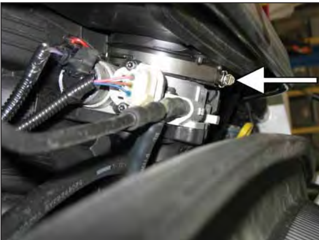
i. Loosen the throttle body hose clamp.
