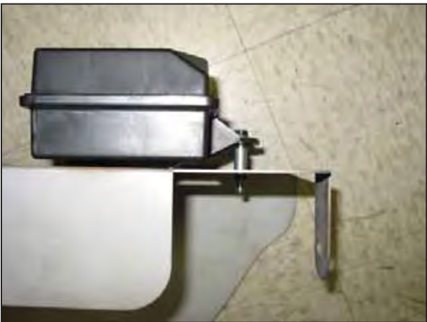
q. If your vehicle is equipped with cruise control, install the vacuum canister as shown. Use the M6 bolt, washer, nipple and M6 nut provided.
