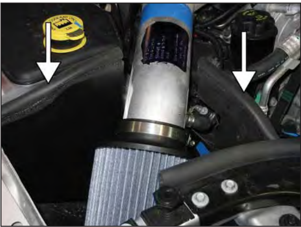
o. Attach foam gasket to the tops of the heat shield.
