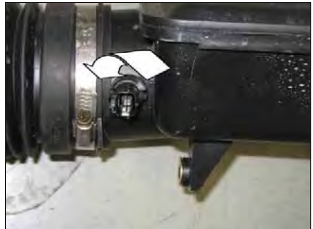
p. Remove the IAT sensor from the stock air box. Turn counter clockwise.
