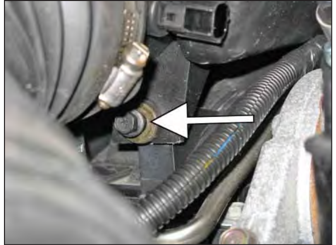
b. Loosen and remove the air box mounting bolt on the passenger side.
