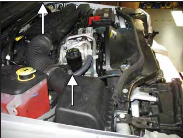
o. Remove the air box assembly.
