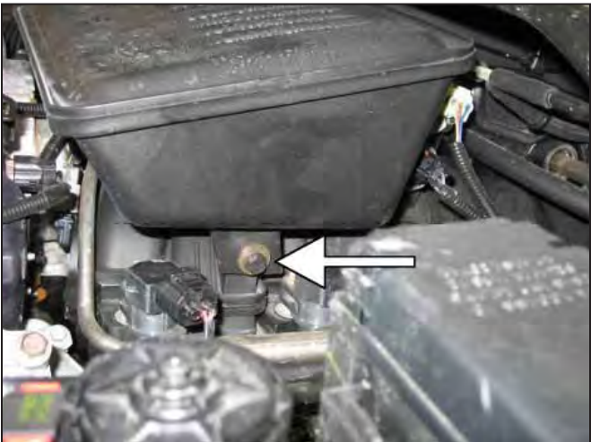
c. Loosen and remove the air box bolt on the driver's side.
