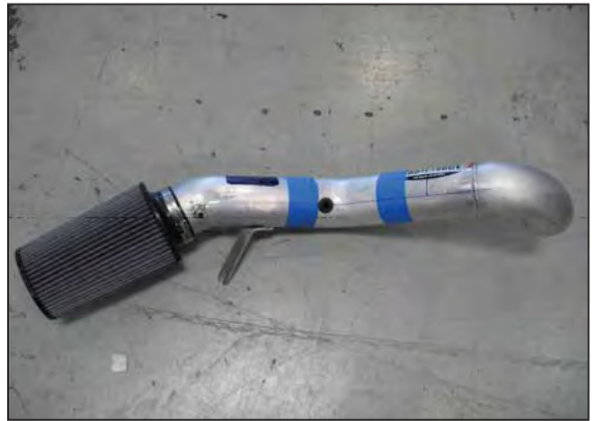
j. Attach the air filter element as shown. Secure with #60 hose clamp.
