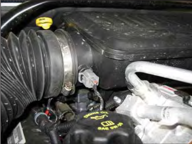
a. Disconnect the Inlet Air Temperature sensor.
