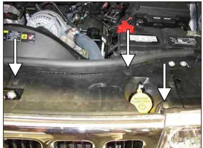
j. Remove push in tabs from the grill. These tabs will be reused.
