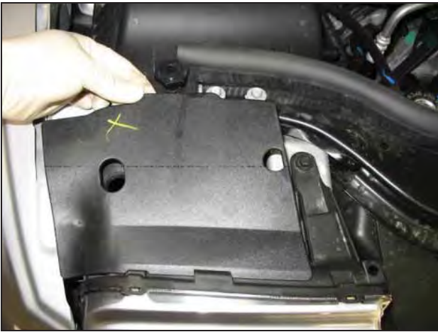
m. Remove the head light cover. Pull the rear up and back
