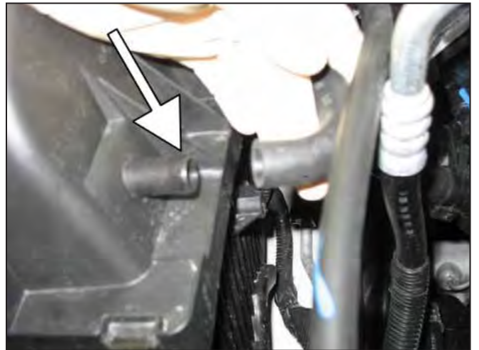
d. Disconnect the crankcase breather hose.
