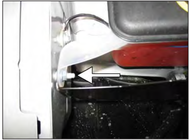
h. Secure the heat shield tab between the fender and the coolant overflow reservoir with M6 washer and nut. Secure reservoir.
