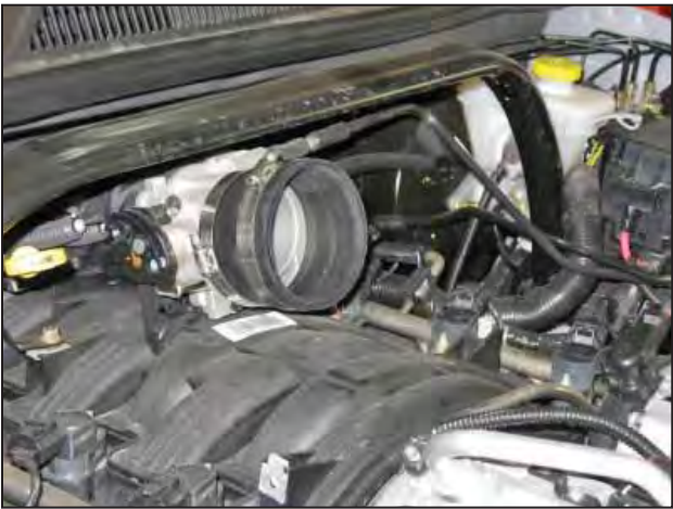
i. Attach the coupler to the throttle body. Secure with #52 hose clamp.
