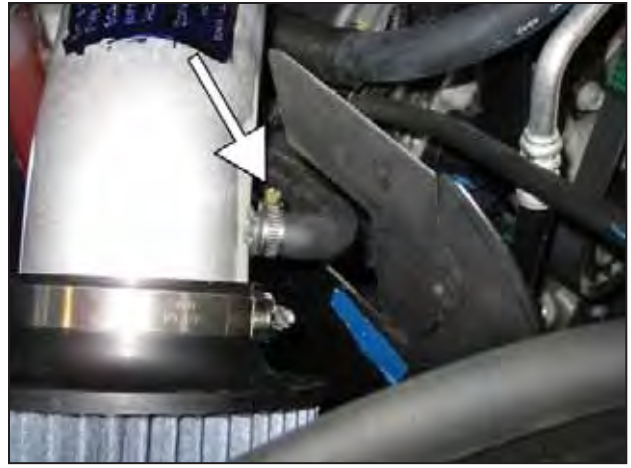
n. Reattach the PCV breather hose and secure with 1" hose clamp.
