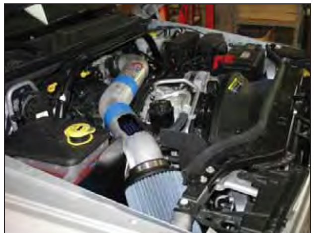
l. Insert the inlet pipe as shown.
