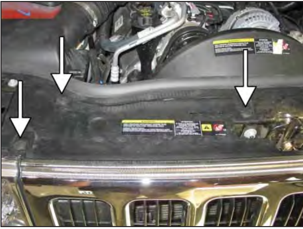
k. Remove push in tabs from the grill. These tabs will be reused.
