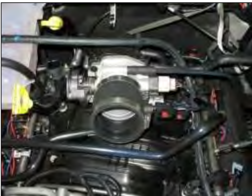
f. Attach the coupler as shown. Secure with #52 hose clamp on the throttle body and #48 on the open end. Reattach the IAT sensor harness to the IAT sensor.
