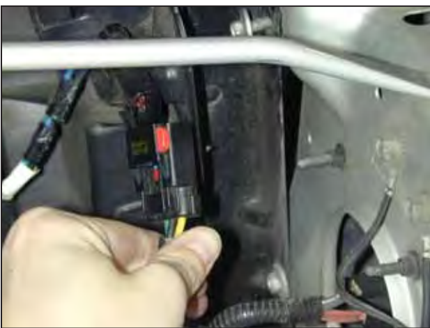
d. Unplug the fan wiring harness from the fan.
