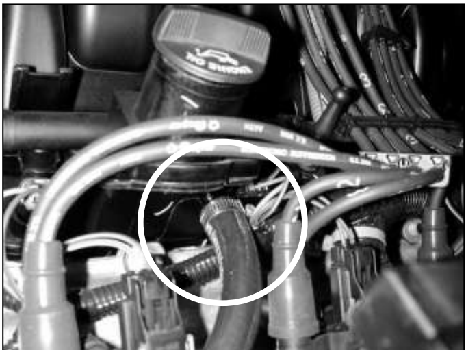
o. Attach breather hose to the factory nipple and secure with provided hose clamp.
