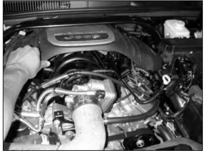
r. Remove oil cap. Insert plastic engine cover and install oil cap. Re-install grill.
