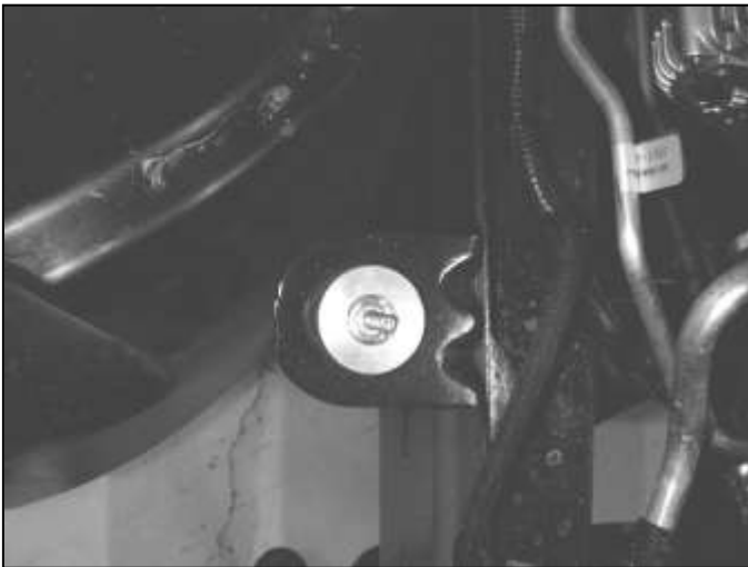
b. Assemble the heat shield mount to the air box mounting tab. Refer to the following diagram, using the 1/4-20 bolt, washer, spacer, and nut. Reuse the rubber grommet from the air box mounting tab.
