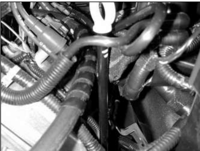
n. Insert breather hose close to the dipstick to provide clearance for the plastic engine cover.
