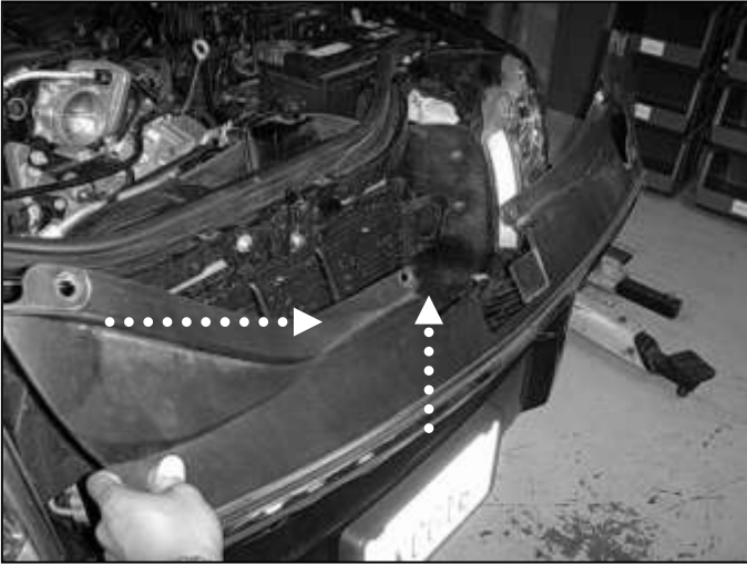
k. With the tabs and remaining mounting hardware removed, pull forward on the grill. Then pull up to remove.
