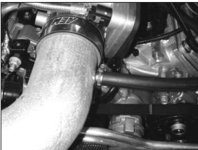
p. Attach the other end of the breather hose to the inlet pipe. Secure with provided hose clamp.
