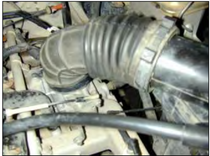
b. Loosen the plastic hose clamps on the rubber intake tube attached to the throttle body. Do this by pulling the two plastic tabs on the hose clamp apart. Disconnect the intake tube from the throttle body.
