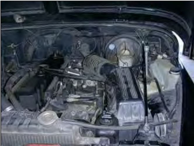
Factory air box system installed
