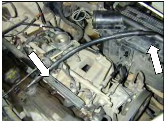
d. Remove the breather hose connecting the valve cover to the air filter housing
