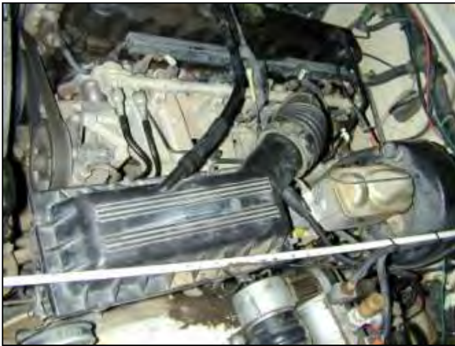
a. Factory air box system installed.
