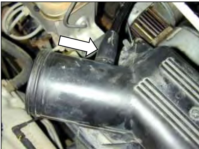
c. Disconnect the charcoal box breather hose from the air filter housing.
