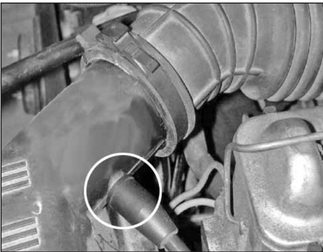
c. Disconnect the charcoal canister breather hose from the air filter housing.
