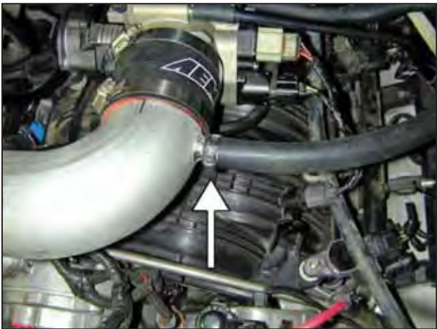
l. Secure other end of the breather hose with provided hose clamp.
