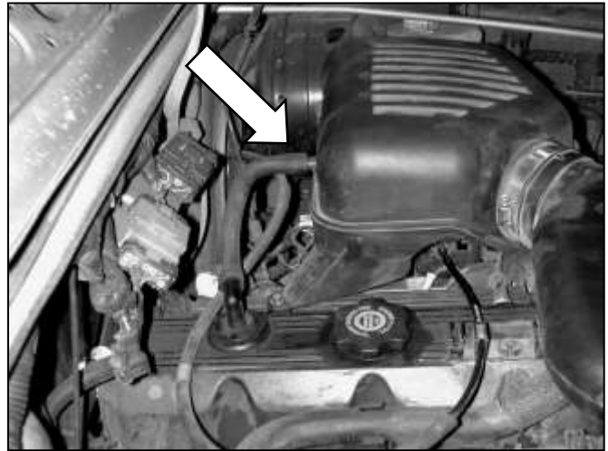
b. Remove the breather hose from the backside of the resonator box.
