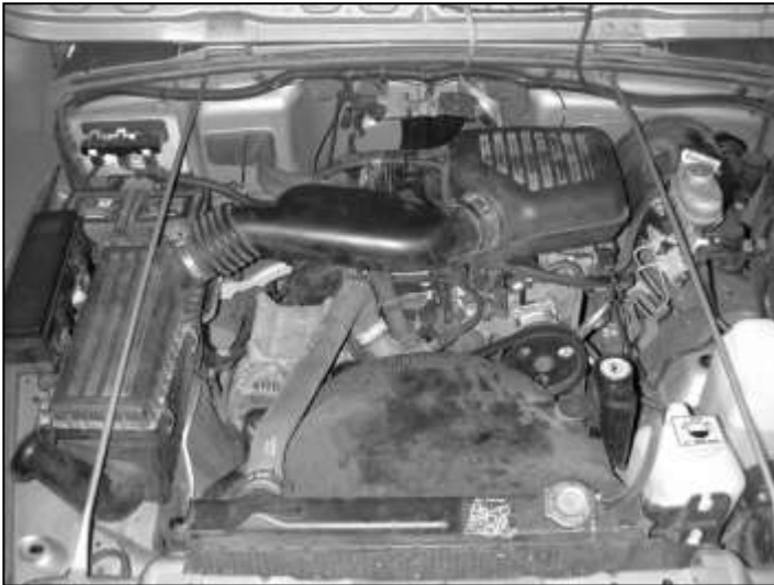
Factory air box system installed
