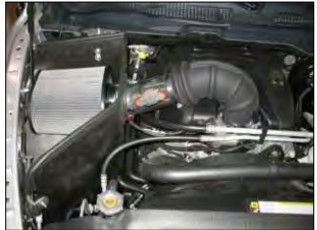
AEM® intake system installed
