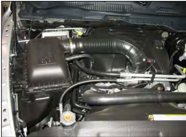
Factory air box system installed
