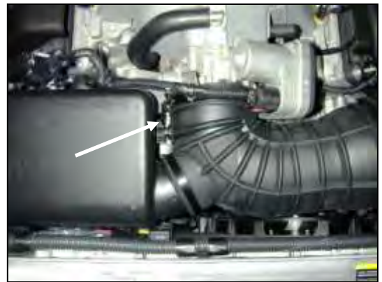
b. Loosen throttle body hose clamp.
