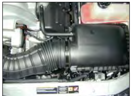
d. Loosen the inlet tube hose clamp. Remove inlet tube.
