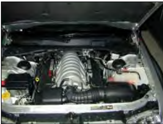
a. Stock intake system installed.
