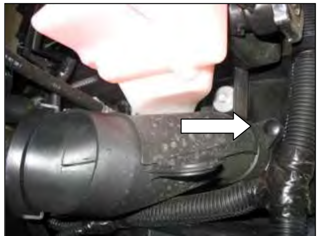
d. Remove the air duct by removing the push-in tab.
