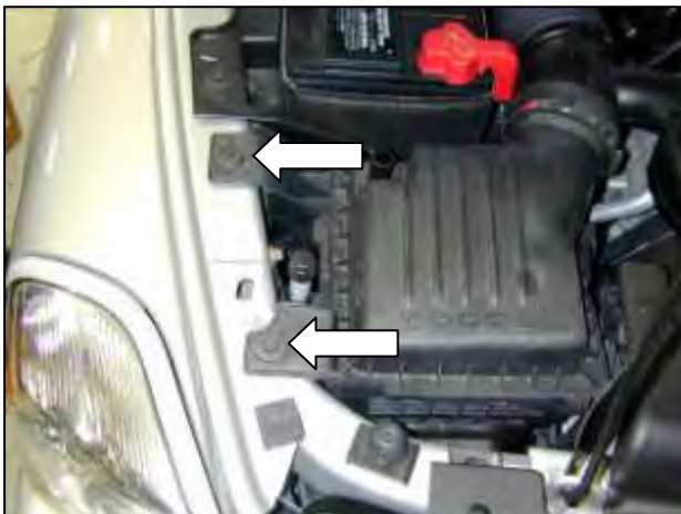
c. Remove the two air cleaner housing mounting bolts.
