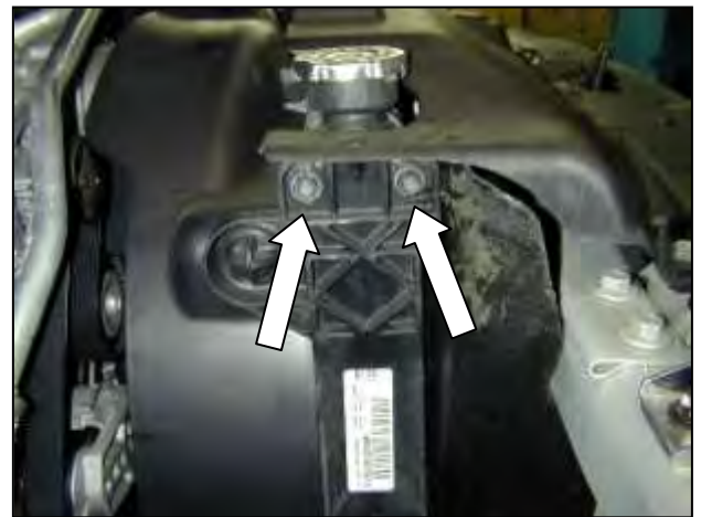
j. Remove the two upper radiator support screws.
