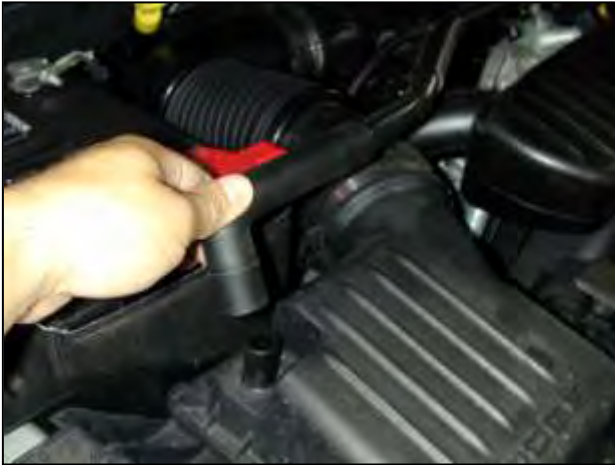
a. Remove one end of the crankcase breather hose from the air box and the other end from the oil fill cap housing.
