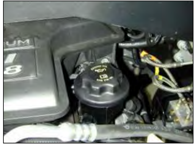
f. Remove the oil fill cap. Put a plastic bag over the opening to prevent parts or debris from falling into the engine.
