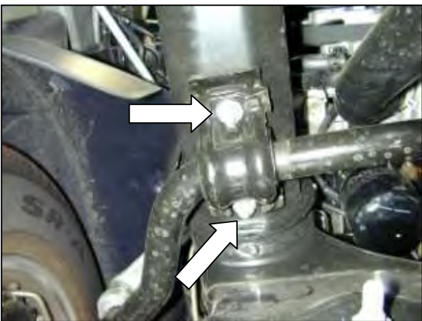
i. From under the vehicle, loosen but do not remove the passenger side sway bar D-bracket mounting nuts. Use a soft-faced hammer to gently tap the bracket bolts up through the frame rail.
