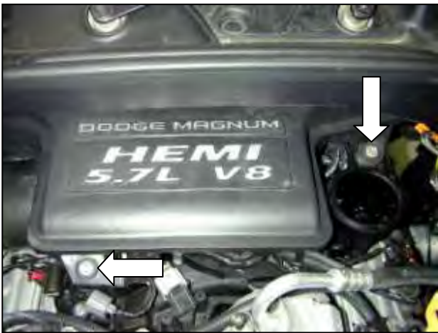
g. Loosen the two resonator mounting bolts and remove the resonator from the engine bay. Replace the oil fill cap.
